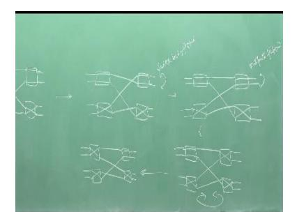
So in this example I have taken remember this is the blocking system this not strictly a non blocking only 2/2 this element this cross bar is a strictly non blocking element but this whole switch per says a blocking system, so a connection for example you want you can set up the connections so I am setting all four of them and trying to figure out the what do you mean by equivalence.
