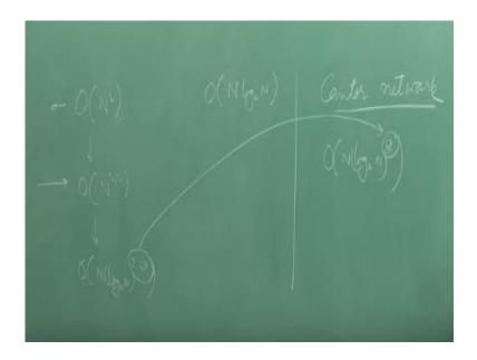
When square which for a cross bar using a Clos network I was able to compute 3/2 by doing recursive construction I was able to come to log to n 2.58 okay while for rearrangibly non blocking switch we actually came up with a cross point complexity of this of course I had already mention that while coming from here to here this was actually strictly non blocking n/n
