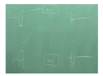
So if you look I actually used demarks this is the 1/N switch okay because 1/M actually where M is  $\log_{2n}$  and there n such switches are used which are 1/m switches then i actually had used these network which is n/n and I had used M such beans network actually and then there was a m/1 switch, n such switches have been used.
