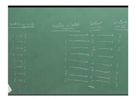
So one will map on to three two will three four to five okay and three will go to two so we will have two one eight four six and seven that is what will be the difference so you can try out various different map center right to find out what will be the content in two different kind of time switches.
