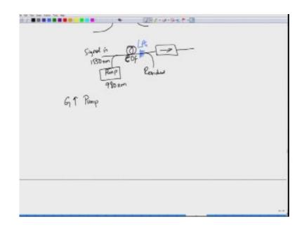
There are couple of things on which the gain depends, we have already seen that the gain kind of increases with the pump power that is input, right so however can it possible that I can just keep on increasing the pump power so that the gain keeps on increasing unfortunately, no. the reason who I does not happen is because a larger number of the pump photons coming in means that these signals are getting excited, okay.
