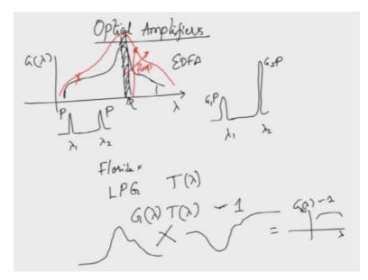
The first thing is if you were to look at the gain of the RBM doped fiber amplifier so you are looking at an RBM doped fiber amplifier, you would actually expect a very flat gain. So over its operating wavelength you would expect it to have a flat gain. Why is this flat gain important? Let us assume that you actually come in with the input signal actually happens to be two wavelengths okay, one wavelength at some  $\lambda 1$  and the other one at  $\lambda 2$ .
