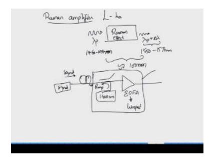
So these are some point about erbium dock fiber amplifier in optical communication recently we have started utilizing another based amplifier called as Raman amplifier the basic idea of a Raman amplifier is very simple suppose I take a photon of some wave length  $\lambda$  p and then I have a medium which has you know which is capable as generating Raman effect okay what is Raman effect.
