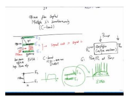
Moreover this requires a WDM pump coupler, pump coupler is a device which actually works something like this, so you have a 1550 nm, which is a signal input power and you have a 980 nm coming from a pump diode and this pump coupler actually couples these two very different wavelengths. So these are called as pump couplers and then you can give this one to the erbium doped fibers for amplification purposes.
