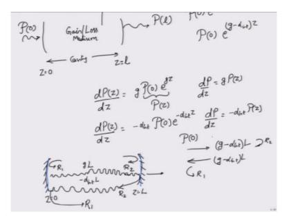
So how the power is actually changing in this gain medium okay, now if of course you can also derive another equation for the loss which is dP/dz will be equal to in case you are only looking at the loss term then  $\alpha_{int}$  will come out and then you still have  $p(0)e^{-\alpha int(z)}$  so another equation that you are going to get will be dP/dz =  $-\alpha_{int}$  times P(z) okay. Now let us look at what is called as a sustaining condition okay.
