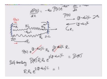
So P(0) times  $e^{g - \alpha int} L$  times R2 would be the power that is reflected which the propagates again as  $e^{g - \alpha int} L$  and then reflects once more to give to R1 okay, this would be the power that is so here you actually have an input power which is p(0) and then after all this round trip propagation and this double reflection you get the power which is p(0) times this particular quantity, of course I can combine this and this into a single exponent.
