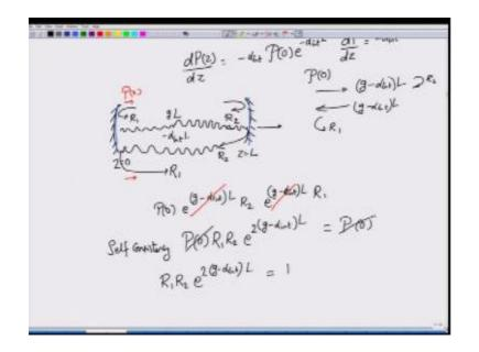
Then you will not be able to get any gain so it simply keeps dropping, dropping, dropping eventually it goes off right eventually it goes to 0 so for oscillations to be sustained it is necessary that this power you know must be equal to the power P(0), from this you can cancel P(0) and then arrive at a relation which is  $R_1 R_2 e^{2(g-\alpha)L}$  must be equal to 1, okay this is the self consistency requirement and you are need to really satisfy this particular condition.
