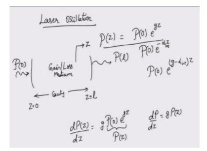
Mechanism freed back mechanism in optics is actually in the form of a cavity the cavity keeps pumping things back and then you have a pump could be a flash lamp in some of the lasers or it could be a electrically pumped signals so you have either an optical pump or an electrically pump the idea of pump is to basically push the atoms from N1 to N2 to create a population inversion okay.
