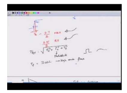
10% to 90% of the final value transition, what is the time required for 10% to 90% transmission and this is called as the rise time of the pulse, okay. For the Nrz this is about 0.7/B, this is for the Nrz case and for the Rz case this is only about half the time, okay, because Rz pulses has to rise up because they also have to fall down, right? In the half period they have to rise and then they have to fall.
