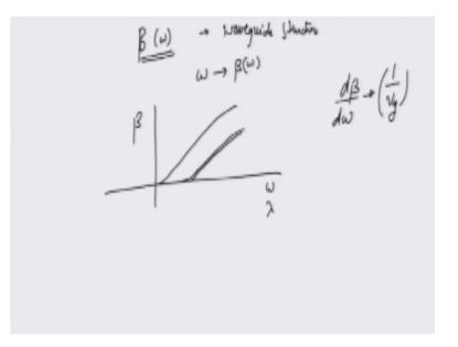
Because  $\beta$  is non liner function of  $\omega$ , now regardless of what kind of dispersion that we are considering, what seems to be clear is that I can consider  $\beta$  as a function of frequency  $\omega$  or
