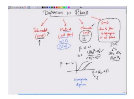
This problem inter model dispersion simply disappears the reason being this is a single mode fiber which means that there is only one mode in which the energy can propagate this would be the  $LP_{01}$  mode or the  $LP_{10}$  mode the XNY modes so they will propagate through the fiber and therefore there is no problem with multiple modes sharing the energy and hence getting some kind of a interference happening at the pulse priding happening.
