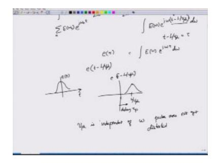
Theory and then see that if this is your e(t)so this is t and this is you time doming function e(t)then the function e(t) - 1/vph is simply the same pulse completely unchanged except that this is delayed by a factor of 1/vph so this is the amount of delay  $\tau$  that you are looking at, this delay incidentally is called as the phase delay  $\tau p$  okay. The important point to note here is that as long as the phase velocity is independent of the frequency right.
