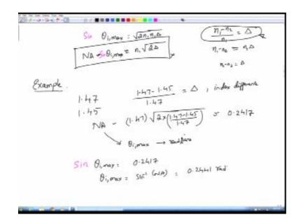
Numerical aperture is still 0.2417 but the acceptance angle is basically sin  $\theta_{imax}$  which should be equal to the numerical aperture 0.2417 from here you can find out what is  $\theta_{imax}$  this is sin inverse of numerical aperture which is sin inverse of 0.2417 and this is roughly 0.2441 radiance.
