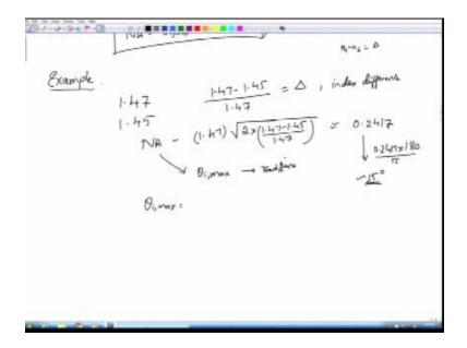
So numerical aperture we have obtained the maximum angle of incidence  $\theta_{imax}$  so we had defined the numerical aperture as  $\theta_{imax}$  we will define not  $\theta_{imax}$  as the.
