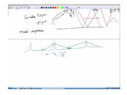
Now what happens is that if you work to send your pulses at a certain rate okay so let us say this is a pulses which are being sent and each pulse carries an information and let us say that time or of between the pulses is  $T_b$  which will be equal to 1/B where B is the bit rate of the system. Okay so you are sending out one bit represented by one pulse here so you are sending out each pulse at a rate of 1/b pulses per second.
