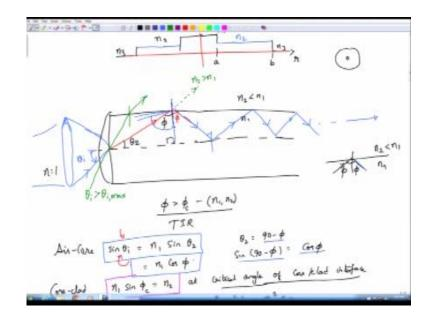
And the core interface so this is basically air Core interface equation, now you have another equation at the core cladding interface right, so this is the equation at the core cladding interface and this equation where we have written  $\emptyset_c$  implies that you are looking at the critical angle of the core cladding interface and critical angle of the core cladding interface is given by Sin  $\emptyset_c$  solving this particular equation.
