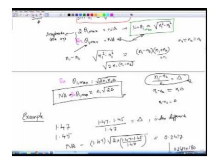
As the numerical aperture but rather sin  $\theta_{imax}$  has the numerical aperture, so if we do that one then what happens is that this is sin  $\theta_{imax}$ , sorry so this is sin  $\theta_{imax}$  a small correction we are not defining  $\theta_{imax}$  as the numerical aperture but rather sin  $\theta_{imax}$  is the numerical aperture, so sin  $\theta_{imax}$ will be  $n_1\sqrt{\Delta}$  and you can, so this has to be slightly change now, so this is NA.
