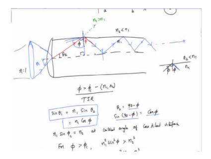
When you shine light on the fiber and you get the light into the core the core cladding interfaced must allow a total internal reflection because when once there is a total internal reflection in the core cladding interface whatever the power that is going from the core will be reflected back into the core itself of course for all angles it will not happen it will only at specific I mean only after a specific angle is reached.
