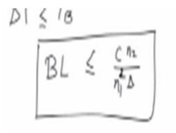
If you want a larger length then you wan t reduce the bit rate, for a given multimode fiber with the parameter n2, n1 and  $\Delta$  known to you, this would be the limit on the bit rate into distance factor. Thank you very much.
