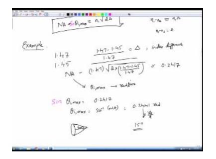
Then this lens has to have an cone angle, okay if you want to put everything into this particular core then the angle of this one should be the cone angle should be 30° nearly, okay.
