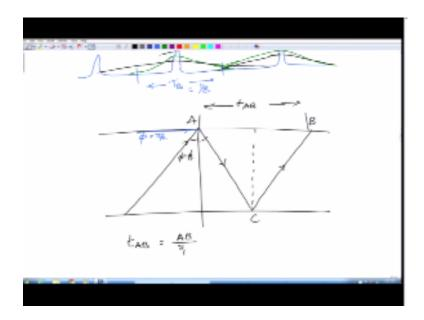
One case is when I have a mode ,which is right at the critical angle incident at the critical angle and one where I have a mode which is incident almost horizontally, okay, so this is when  $\varphi = \varphi/2$ , and this will; horizontally incident ray of light will actually transmit, okay, I mean it will go back.
