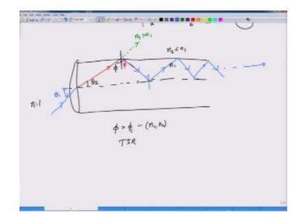
And since b is sufficiently large it does not really contribute much to the propagation so it is only N1 N2 and a that are primarily very important for the calculation of the optical mode. Now what I will do is in the next five minutes give you very, very simplistic view of how a mode is propagated inside an optical fiber. Let us assume that this is the optical fiber this has a nice syndical cross section and there is an axis of the cylinder along like this okay.
