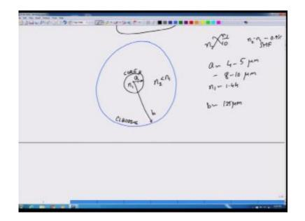
A typical single mode fiber will have a certain core radius, okay this is around 4 to 5 micron core radius and the diameter is about 8 to 10 microns and then it is also topped with certain materials the basic material is silica but it is topped with certain materials in order to raise its refractive index to n1, so let us call this as refractive index n1 and let us call the core radius as a, so this a is typically 4 to 5 micron making the diameter as a 8 to 10 microns.
