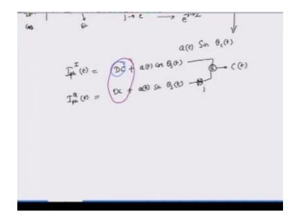
So I don't have to retain the Dc signals for my in phase and quadrature components, so I will directly able to obtain the in phase as well as quadrature components without having to deal with the DC problem. One final point we have obtained in phase as well as quadrature components, this is called as IQ demodulator or IQ receiver, because we're subtracting two photo currents in order to eliminate the DC, this is called the balance photo detection.
