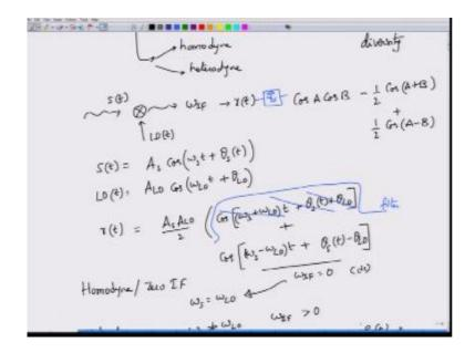
Where we consider the heterodyne receiver you had the output which was  $\cos(\omega s \cdot \omega lot + \theta s(t) \cdot \theta loc$ where  $\theta lo$  was the phase of the local oscillator which if you remove it will then become exactly equal to the signal that you have obtained in this case, so what you have done is to take two optical signals. (Refer Slide Time: 15:23)
