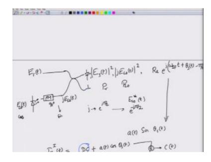
So I take the incoming signal as it is which is  $E_s$  (t) and then put it through the coupler but instead of sending this signal from the local oscillator directly coupling it to the directly to the coupler what I do is I send it through a phase modulator okay I send this through a phase modulator and set the phase modulator such that it provides 90<sup>0</sup> phase which means that instead of  $E_{lo}$  (t) going in to the coupler what you get is  $J_{elo}(t)$ .
