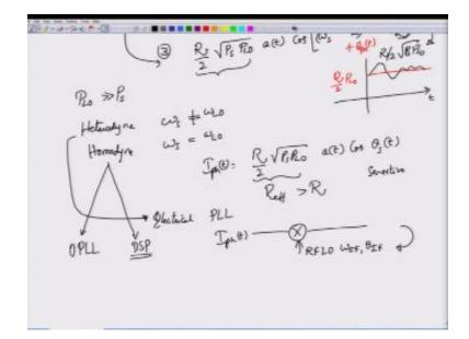
This is the technology that is currently being used so we use high speed DSP is in order to estimate the phase of the incoming signal in order to perform carrier recovery as well as for incarnating or local oscillator with the incoming signal. Okay something that we will talk about it in the later in the course okay we have talked about the coherent receiver homodyne one thing you might have notice is that this photo current that we have obtain.
