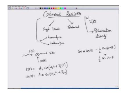
S(t) will be multiplied by a local oscillator call this as some Lo(t) okay and then the resulting signal is proceeded further if the incoming signals frequency is different from the local oscillator frequency then you end up with what is called as a intermediate frequency your spectrum will be centered at the intermediate frequency otherwise the spectrum will be centered at 0 intermediate frequency o intermediate frequency is nothing dc right.
