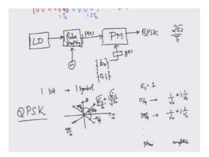
To Implement this one all I need to use is a laser diode I need to have some signal source so I use a laser diode the output of the laser diode can be pulse shaped so I use a pulse shaping MZM so to the pulse shaper I might supply an RF signal so that I get a 33%, 67% or 50% output optical pulse shapes, right. Once I get the optical pulse shapes I just have to use a phase modulator whatever the bit sequence that I am getting here BN which can be a sequence of 01 right.
