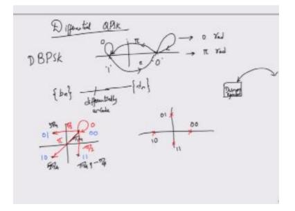
So in the next case, I can write this s 0 phase, I can even transmit that corresponding slot s 0 phase shift at sequel, so similarly you have to have a dummy symbol, let say the dummy symbol for differential QPK signal is 00. So the ways to implement this one will be the same and we
