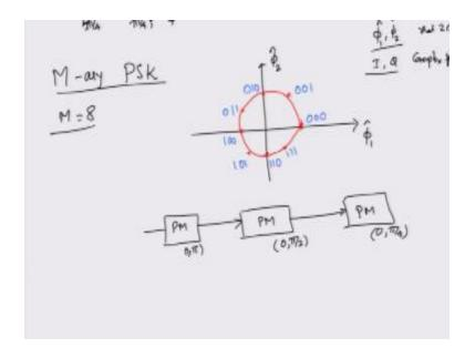
So if you use a bit sequence and then put a de multiplexer over here, and then sending the MSB bit to the first phase modulator, from the middle bit to this one and then send the LSB bit to the last phase modulator, you can see that the total phase that you will obtain in will be a linear combination of all these three and it will then implement this. Thank you.
