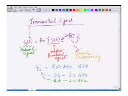
Now, let us look at the transmitted signal the transmitted signal in the wireless communication signal system. The transmitted signal can be written as follows what we call as a pass band signal Sp(t) equals –
