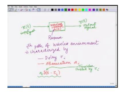
Let say we have a signal x(t) which is input to my signal to my wireless system and this is my output signals. This is my input signal and this is the output signal and this is my wireless environment or my wireless channel between the transmitter and receiver, you would like to develop a model for the response of this system that is h(t) impulse response of the system, we would like to develop a model for the response of the system this is also known as the wireless channel.
