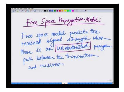
So, let us start with the basic model which is the free space propagation model. So, I want to start with the basic model which essentially the, which is the free space propagation model. The free space propagation model it predicts the receive signal strength when there is an
