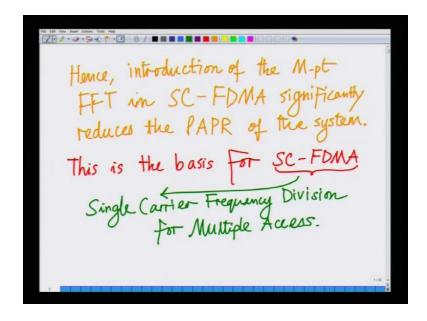
Hence, hence introduction of this M point FFT significantly reduces the PAPR of the M point FFT in SCFDMA significantly reduces the PAPR, significantly reduces the PAPR of the system. And this is essentially transfer this is essentially the techno this is essentially the SCFDMA scheme, which is single carrier FDMA. Hence, this is the basis SCFDMA where SCFDMA as we have talked about stands for single carrier frequency division multiple. This
