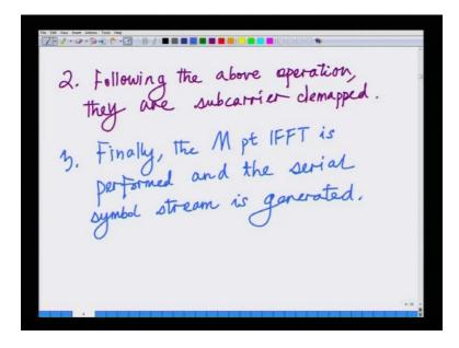
They are subcarrier de-mapped, this is essentially inverse of the mapping operation that was done at the transmitter. Remember earlier the OFDM transmitter schematic, we had a subcarrier mapping operation. Now, we have a de-mapping operation at the receiver. Finally, the IFFT is carried out and the serial symbol stream is generated. Finally, the M point IFFT is performed and the serial symbol stream. Finally, the M point IFFT is performed and the serial symbols is generated.
