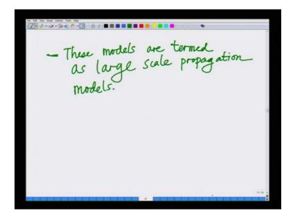
Hence, these models are termed as channel models or large scale propagation models these models. Models are termed as large scale propagation, these models are termed as large scale propagation model, we will start looking at some of these propagation models to characterize the received signal strength in a wireless communication system.
