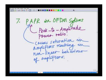
The next we said another important factor that needs to be considered in OFDM is the PAPR in OFDM systems were PAPR stands for peak to amplitude. PAPR stands for peak to amplitude power ratio in OFDM and this also we said causes saturation in amplifiers, causes saturation causes saturation in amplifiers resulting in non-linear behavior, resulting in non-linear behavior of amplifiers in the OFDMA systems. So, that is the problem of PAPR.
