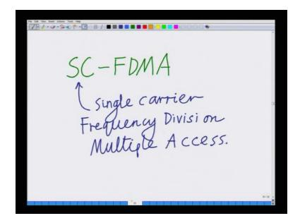
The solution we said is to used single carrier FDMA and that is as follows that is if you observe the OFDM transmitter schematic, if I introduce an N point FFT. Before the N point IFFT the FFT and IIFT cancel and this reduces to a single carrier system, which PAPR is very low. It is almost close to 0 d b that is what we said. Hence, what I want to do is I want to introduce an FFT block before this IFFT. However, I do not want to do an N point FFT
