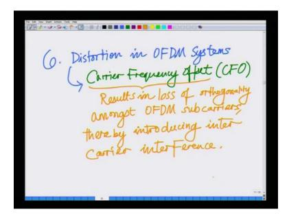
Then we looked at distortion in OFDM systems. We looked at distortion in OFDM systems, namely we looked at the problem of carrier frequency offset offset or CFO which arises in OFDM. This is serious problem we said because this results in loss of orthogonality amongst of d m subcarriers there by introducing inter symbol interference inter carrier interference. There by introducing inter carrier interference.
