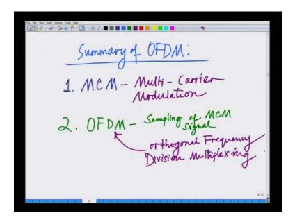
Hence, there are two techniques; one is interleave the 0 this is termed as IFDMA, the other is 2 0 pad, this is termed as LFDMA. In fact this is used in LTE, which is the fourth generation wireless communication standard. So, this brings us to the conclusion of section on OFDM. Hence, let us now summarize the different modules that we have seen in OFDM. Now, let us look at the summary of the OFDM modules that is summary on what we have seen in OFDM so far.
