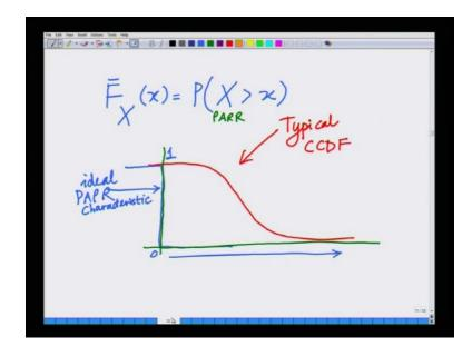
And we also saw that the peak to average power ratio can be measured by this CCDF that is the probability, that the peak to average power ratio is greater than a certain threshold. We also looked at examples for different of how the PAPR CCDF curve looks for different numbers of subcarriers.
