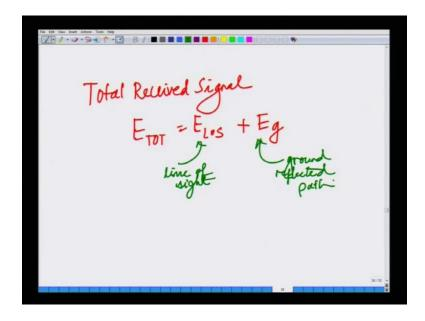
Hence, the total received signal is nothing but e total which is equal to E line of side plus E ground. This is again from the line of sight path and this is from the ground reflected. This is from the ladder sight path and the ground reflected path. Now, each signal E naught first for instance, let us look at the line of sight path that is some E naught
