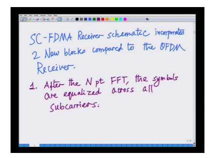
So, this SCFDMA are so s c f d m a receiver schematic. Incorporates two new blocks compared to the OFDM compare to the OFDM after the after the N point FFT the symbols are equalized. So, first N point FFT, the symbols are equalized across all they are equalized across all subcarriers. Then they are subcarrier de-mapped following the above operation.
