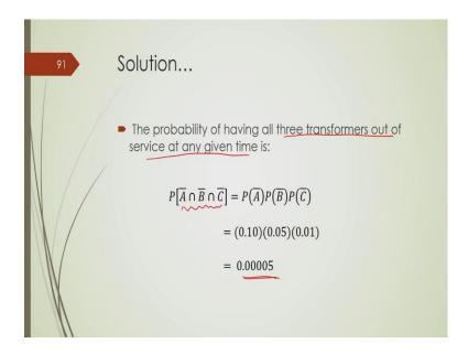
Now what would be the probability of having all the three transformers out of service at any given time which is equal to this probability or this as you know this intersection of these three events where A prime B prime and C bar or A bars B bar and C bar they represent the failure event of individual transformer. When this happens simultaneously so this probability is equal to this ok.
