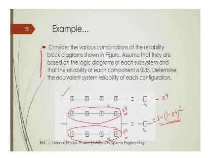
Now, we have some examples, this is easy example only you need to determine that composite reliability or equivalent reliability of several subsystems connected in different fashion. For example, here 4 units are connected in series. So, composite reliability R equivalent will be equal to R to the power n, sorry here n is equal to 4. So, we can directly write as R to the power 4 ok.
