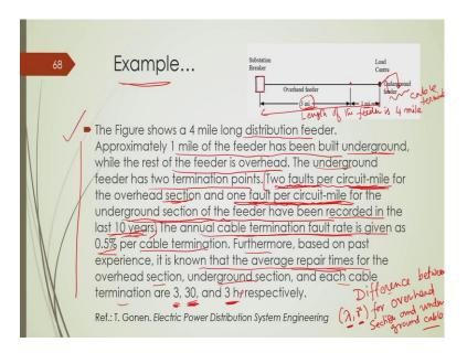
So, look at this example ok. This example is very simple example, we have a substation at this point, and this box is representing a substation or substation breaker ok. And there is a primary feeder, there is a primary feeder and this feeder is of 4 miles of length. So, length of the feeder is of 4 mile; length of the feeder is 4 mile out of which some part is overhead feeder this 3 mile is, some part is overhead feeder and some part is underground cable.
