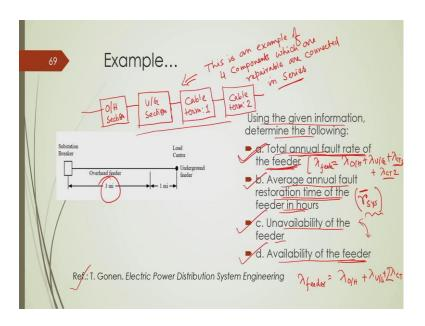
Now, using this information you are supposed to determine the total annual failure rate or total annual fault rate of the feeder i.e., question number a, question number b is average annual fault restoration time of the feeder. And question number c is unavailability of the feeder, and question number d is the availability of the feeder. This problem I took from Gonen's book ok, and this once you got this unavailability, availability is just 1 minus that unavailability.
