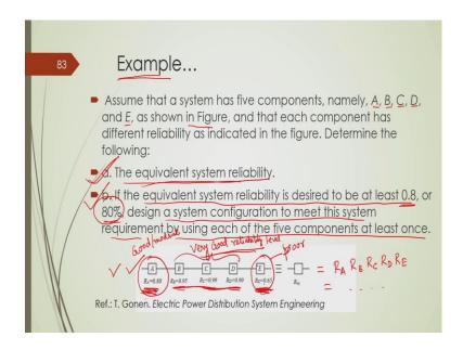
Now we have another example; we have another example. This example says that we have five components A, B, C, D and E they are connected in series combination like this, A, B, C, D, E ok. And their individual reliability value is also given R A is equal to given 0.8, R B is equal to given 0.95, R C is equal to given 0.99, R D is 0.9 and R E is 0.65.
