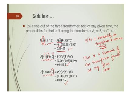
Now, what would be the failure if we have one fault of individual transformer at a time. So, if we have you know one fault at a time. So, this event is translated as A prime. So, probability of A is basically representing this reliability of the system that is probability for transformer A not to fail not to fail ok.
