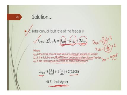
So, we write it in the next page that this here OH represents this total annual fail fault rate of the overhead section, this lambda UG represents that total annual fault rate and of the underground section and lambda CT is representing total annual fault rate of the cable terminations ok. Now, if we know these values of this lambda OH, lambda UG and lambda CT, we can find out the total annual failure rate or fault rate of the feeder ok.
