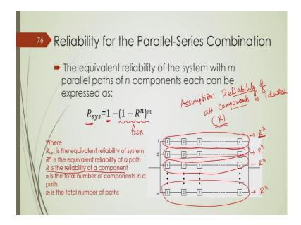
So, this we will make a series parallel combination ok. So, let us consider we have here n number of equipments which are connected in series and this will constitute 1 unit, this is one unit and there are. So, this is unit 1 and there are you know m number of such units. So, we have n number of subsystems they are connected in series and which constitute 1 unit of the system.
