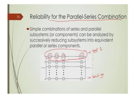
Now, we will determine that reliability for a parallel series combination ok. So, as I said in a practical power system, there may be a several components out of which some are connected in series and some are connected in parallel.
