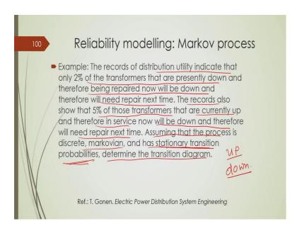
So, I have a small example which would be useful to understand the concept that a distribution utility having a 2 percent of transformers that are presently down and therefore, being repaired now will be down also and therefore, we will need to repair next time. So, there are 2 percent transformers which are presently down and after repairing there is a probability that they will be down ok.
