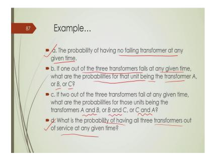
So, based on this information determine the probability of having no failing transformer at any given time, that is basically the reliability level of the overall system having three transformers. Second is if one out of these three transformers fails at any given of time what would be the probabilities of that unit being the transformer A, transformer B and transformer C; that means, what is the probability of the failure of individual transformers A, B and C ok.
