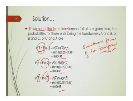
Similarly, if we have simultaneous failures of the transformer, so here this is the example of simultaneous failure of two transformers ok. So, we have two transformer failed at a time that is A and B, C is healthy ok, here we have two transformer B and C are having this failure where A is healthy, and this is the case where this A and C are will encounter faults simultaneously when B is healthy ok. So, individual probability you can find out alright.
