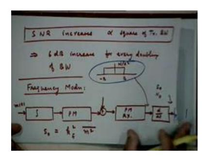
So, SNR increases and delta omega in some sense is the measure of the bandwidth of the message signal is in it because actually bandwidth is delta omega plus 2 by B, delta f plus B. So, if you assume that this much smaller than delta f, so delta f is the measure of bandwidth in some sense, so larger the bandwidth of the phase modulated signal the larger the improvement or better the output SNR, so that is the key result here.
