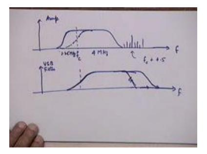
So, if you want to draw the spectrum of the transmitted signal, this is what it will look like. So, let us say this is your f sub c this is one side of the upper side band of the picture signal DSB mod DS amplitude modulation, the lower side is transmitted the low the lower side band is cutoff.
