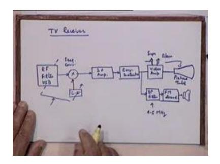
Next we come to the receiver, I am sure you can draw the diagram yourself, so you start with the RF filter which has those characteristics that I just mentioned. It is also a VSB filter, along with other functions it also carries out the VSB filtering or VSB shaping function spectral shaping function plus, of course it provides the required amplification.
