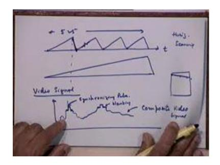
Let us look at we also saw very briefly the scanning pattern, the horizontal scanning pattern and the vertical scanning pattern. Let me just repeat that once again this is the saw tooth waveform which depicts the way, the scanning is done left to right that is the horizontal scanning, this shows horizontal scanning and this shows vertical scanning. Of course, I should show a break here, because there will be 525 such horizontal scans corresponding to one vertical scanning
