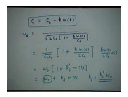
So, basically what we are saying is that the capacitance C of this kind of device varies something like this, it oscillates or it varies around some fixed values of the capacitance. So, C sub 0, C sub o is the nominal value of the capacitance without application of outside voltage and as we apply an external voltage it varies in this manner. So, if this is the message signal and you apply this across the reverse bias junction, this will create a junction capacitance which has...
