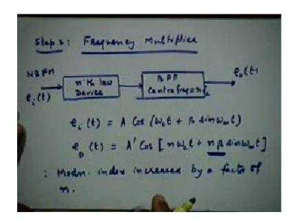
So, that step of converting a narrowband FM into a wideband FM has to be carried out by what is called, so this is step 2 the frequency multiplier, a frequency multiplier precisely there is an operation I just mentioned. Now, that is, it multiplies the argument of the cosine sinusoidal function by certain factor. Now, again there are certain ways of utilizing a frequency multiplier, I will discuss one of them at the moment which you are familiar already.
