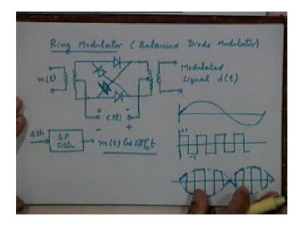
And that is precisely done by a device called the ring modulator or the balanced diode modulator, the typical circuit will look something like this, this should have been like this, so this is the balanced modulator, it is also called ring modulator. The reason being that these diodes all face in the same direction, as we trace the diodes their all point in the same direction. So, if you go along these diodes they form a ring in some sense, so
