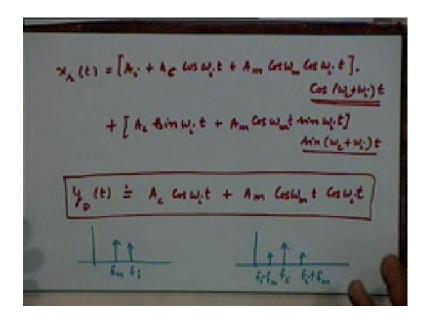
You get x sub r t is equal to A sub i plus A sub c cosine omega i t plus A m cosine omega m t cosine omega i t into cosine omega c plus omega i t plus A sub c sine omega i t plus A sub m cosine omega m t sine omega i t into sine omega c plus omega i t. So, once again I have quadrature representation, so please assume this is correct this is just coming out of, important thing is instead of writing it in terms of quadrature representation using omega c I used omega c plus omega i.
