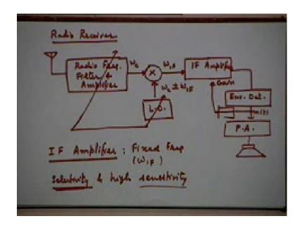
So, the super heterodyne receivers precisely does that, you have your signal coming in from the antenna, the first stage has to be, the radiofrequency stage, which carries out initial. This is the radio frequency filter and may be some amplification, remember filtering has to be done for 2 reasons, one to reject, other signals and the other the remove noise out of band noise.
