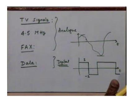
So, we will return to this point later if required, now let me briefly talk about some picture signals. The two kinds of picture signals that we have talked about is the TV signal and the facsimile signal, the TV signal is a moving picture signal. So when it is a moving picture signal, you have to make sure that you do not reduce the essence of motion itself. So, typically as I said you have to first convert this signal into an electrical
