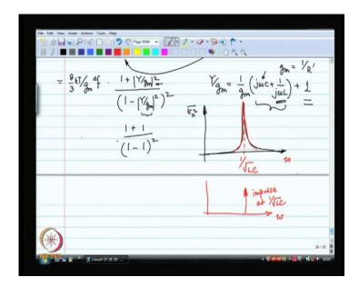
So, what you had hoped for was the spectrum of the oscillator to look like an impulse this is what you wanted to make instead because of noise channel noise in the mosfet I did not even talk about noise in the resistors right. But There is going to be noise in the resistor there is no real resistor over there its a resistor because of the loses in the inductor, but that will create noise loses in the inductor means that you have got noise over there anything which is lousy will have noise.
