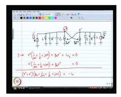
So, I have got L to ground R prime to ground and c to ground c is not really the actual capacitance it is the capacitance insant with all the parasitic capacitance I have got another c another R and another L all of these are to ground. and I have got this noise current source on the both sides as well alright. So, this is my complete small signal model and the way we deal with noise is that we take 1 source at a time and we add the effect of both together at the output.
