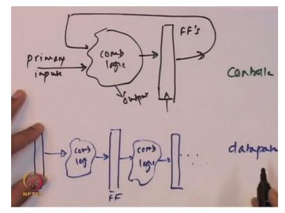
There is a controller, a controller is basically a set of flip-flops which maintain the state and combinational logic which will generate the next state based on the current state, these flip-flops maintain the current state and there is a clock and this combination logic is computing the next state which is to be loaded into the flip-flops at the beginning of the next clock cycle or the end of the current clock cycle.
