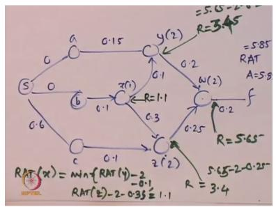
Somehow maybe a coincidence but like actually it is not, over here we have found this required arrival time at the output of z to be 3.4 which is same as the actual arrival time at the output of z, which is 3.4 but the AAT at output of y is 3.2 but the required arrival time at the output of y is 3.45, so there is a discrepancy here and there is like you know thing matching over here. Anyway, so just you would have probably guessed the reason for that also.
