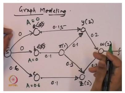
So I will just draw the graph first, recall that there are a, b and c, there are this primary inputs or it could be secondary input, but inputs and there were labels here, 0, 0 and 0.6, okay. So this label we are denoting the arrival times of signal transitions at this input, so I am going to have some kind of dummy source and arcs of this kind, directed edges of this kind and this I am going to label with this.
