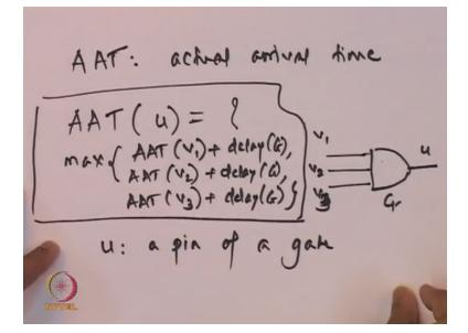
So this concept of actual arrival time, so actual arrival time at U say where U is a pin of a gate, okay, say it could be output or input pin, so this actual arrival time at a you at a pin U say U, this is a gate and this is say U okay, so how is it going to be defined and what will determine this particular actual arrival time, which is the arrival time of the signal transition.
