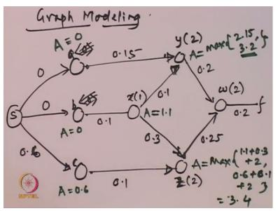
So topological order here will be first we will do x, because x does not depend on once we had done a, b, c, x can be done immediately but neither y nor z or w can be done because they will depend on x, so what will be the arrival time of the signals transitioned at the output of x, A at this point will be see that because of this path 0+0.1+1, 1.1, there is no other way output of x will be influenced. So it is 0+0.1+1, 1.1, so A is decided over here.
