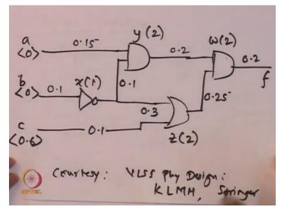
The signal is arriving here at times 0 so based on this can we decide what would be the arrival time of signal at the output of y, not exactly I mean we know this information, this 0.15 +2 but this signal transition here to a final value possibly could depend on some other input path. For example, it could depend on a signal going along this wire getting delayed here, getting converted and other delays.
