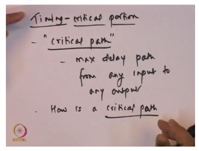
And that is of course crucial because this notion of critical path that I mentioned which you are really familiar with which says, it is max delay path from any input to any output, but that any input, any output include not just primary input, primary output but also this secondary input, secondary output which are respectively the flip-flop outputs and flip-flop inputs, okay.
