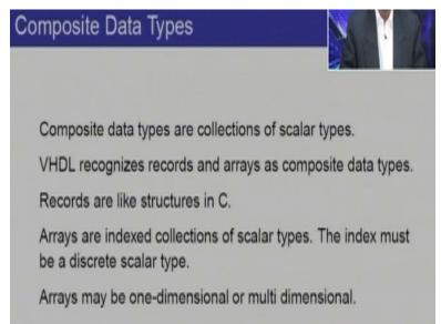
Having done the scalar types let now look at composite data types, these are the types which consists of a base unit type and then what we declare is a collection of composite types, so composite data types are collection of scalar types, VHDL recognizes records and arrays as composite data types. Records are like structures in C, they permit a collection of heterogeneous kinds of scalars. Arrays are indexed collection of scalar types.
