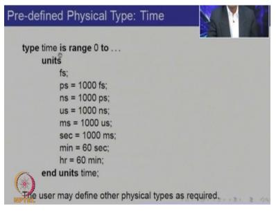
This is the pre-defined type physical and the pre-defined unit is femtoseconds, so you can say type this is how it must have been described internally, it is equivalent to a definition of this kind, type time is range 0 to some maximum value, then you have a declaration units and the base unit is declared first, this one is compulsory others are optional. So the base unit then is femtosecond.
