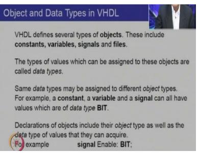
We had also seen object and data types, object types are constants, variables, signals, files and in fact that are pointers types as well and then the data types could be of type bit, of type std logic define later in library and so on.
