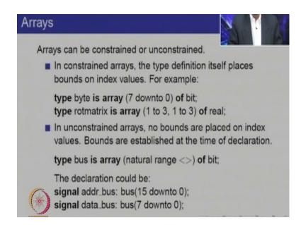
Arrays are particularly important and they can be constrained or unconstrained as we had seen earlier, in constrained arrays the type definition itself places bounds on index values, for example we might say type byte is array 7 down to 0 of bit or type rotation matrix rotmatrix is array 1 to 3, 1 to 3 of real, so it is a two dimensional array for a rotation matrix which will have sin theta, cos theta, sin pi, cos pi kind of entries therefore those are real.
