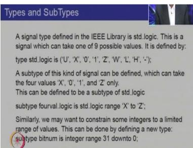
Now notice that for each type you can define a subtype which does not use all the possible values defined in the main type, for example if you use the IEEE library it defines a new signal type called std logic which is quite commonly used, std logic is a signal which can take one of 9 possible values, it is defined by a statement of the type.
