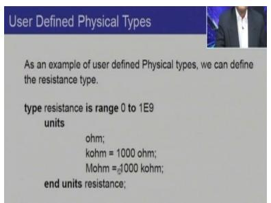
Just to take an example, let us say we want to define a new type new physical type called resistance, we can declare it as saying type resistance is range 0 to 1E9 with units ohm that is the base unit and derived units which are Kohm or kilo ohm equal to 1000 ohm and Mohm or
