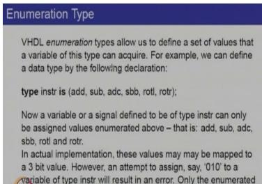
So enumeration type allows us to define a set of values that a variable of this type can acquire, for example we can define a data type by the following declaration, the keyword type must be used first so you say type instr instruction is and then you give a list of values which are enumerated, so for example I might say type instruction is add, subtract, add with carry, subtract with borrow, rotate left, rotate right, this limited set of commands now has been enumerated.
