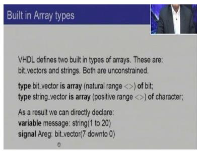
There are as we had said earlier built-in array types, where bit vector is an unconstrained array of bit and string is an unconstrained array of character, as a result you can directly declare variables or signals of this kind for example you might have a declaration which says variable message is a string 1 to 20, notice string is an unconstrained array of characters and here we are saying that message will be a collection of 20 characters whose index will go from 1 to 20.
