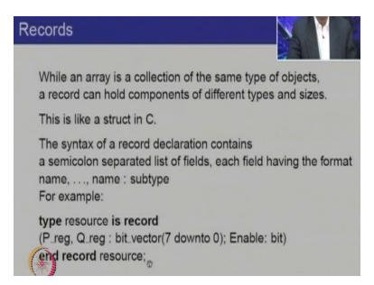
Records are on the other hand collections of different types, so while an array is a collection of the same type of objects, record can hold components of different types and sizes, this is like a structure in C. And the syntax of a record declaration contains a semicolon separated list of fields, each field having the format name name name subtype.
