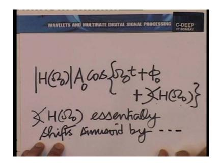
What is the effect of this angle? As you can see the effect of this angle is to change the phase and a change of phase is equivalent to a change in time. So, it is like shifting the
