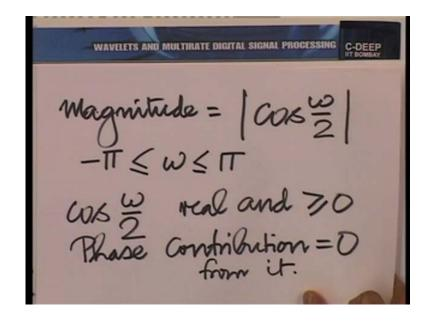
So, the magnitude of this response would be mod cos omega by 2 and let us confine as I said omega between pi and minus pi where upon cos omega by 2 turns out to be non negative. In fact, essentially cos omega by 2 is real and greater than equal to 0 in this region. Thus, phase contribution for this term is 0. Say, if you look at the overall frequency response here, namely e raise the power minus j omega by 2 times cos omega by 2. This has no phase contribution.
