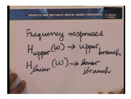
So, if you call the frequency responses of the upper branch and lower branch, respectively as H upper omega and H lower omega. Upper branch, lower branch. Then two properties are immediately satisfied.
