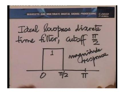
So, an ideal low pass discrete time filter with a cut off of pi by 2 would look something like this. I mean in the magnitude sense. So, it would have a magnitude response that looks like this and ideally, the phase response would be 0. So, it would be 1. The response itself would be 1 between 0 and pi by 2 and 0 between pi by 2 and pi and of course, mirrored as it is between minus pi and 0.
