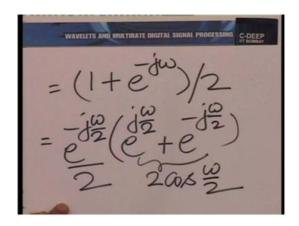
That would give us 1 plus e rise the power j omega by 2 minus j omega by 2. If you like which we can simplify, we can take e raise the power minus j omega by 2 common here and then put e raise the power j omega by 2 plus e raise the power minus j omega by 2 inside the bracket and leave the half factor as it is.
