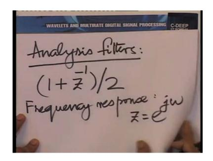
Indeed, consider the analysis side and the analysis filters, both of them have a frequency response obviously. Let us take the filter 1 plus Z inverse by 2 and let us look at its frequency response. Of course, we would obtain the frequency response by substituting Z equal to e raise the power j omega.
