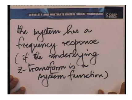
The system has a frequency response. That is you see we talk about the system having a frequency response if in the underlying Z transform is a system function. If the underlying Z transform is a system function and of course, otherwise in case we are talking about a sequence, then we say the sequence has a discrete time fourier transform.
