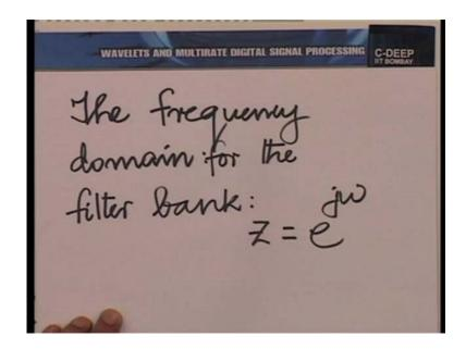
Now, our objective here is to look at the frequency domain behaviour and how would we get a frequency domain representation of the Haar filter bank. So, what we will do is, we will progress follows first we shall look at the frequency domain for the filter bank. How would we do that? We would do that by substituting Z equal to e raise the power j omega.
