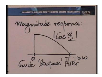
Now, when an impulse response is real, the frequency response is conjugate symmetric. So, whatever is the omega is also at minus omega in magnitude. Whatever is the omega in phase is the negative of what is there at minus omega in phase. So, we need only to sketch the magnitude response and the phase response between 0 and pi. We can ignore minus pi to 0 because there is going to be conjugate symmetry.
