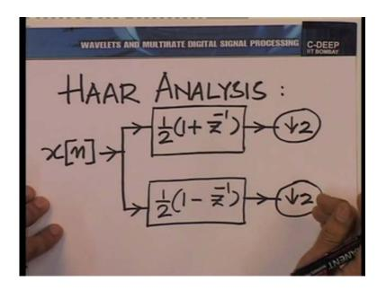
So, I just put down the two filter banks. Clearly, you will recall that on the analysis side, we had a structure like this. We had the sequence, let us call it x of n corresponding to this to the function in V1. Essentially, it was subjected to the action of two filters. A filter of the form half 1 plus Z inverse, another one of the form half 1 minus Z inverse followed by a down some link by 2.
