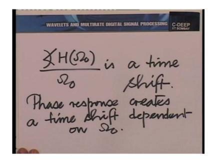
Now, just in case it is independent of omega naught, we have a good situation. So, you know this time shift actually is what is called a necessary evil in the frequency response. You know most of the time when we give specifications for designing a filter, whether it is in the angular domain or in the discrete time domain, we do not really want the phase response. The phase response comes as a necessary evil and we have to work around it.
