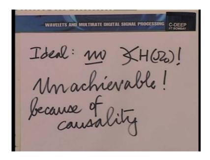
Incidentally, that is why you can 0 phase filters in dealing with images in dealing with two dimensional data because in two dimensional data, causality is not an important requirement but when you are dealing with one dimensional data in time, causality is essential. You cannot avoid it and therefore, you cannot avoid a phase response either.
