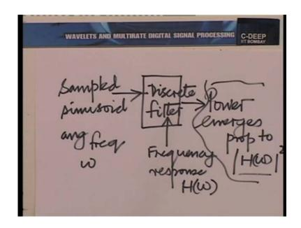
Let us say the angular frequency is omega and the frequency response here is H of omega. Then the power that emerges from here is proportional to mod H omega squared. So, in other words, whatever is the power of a sample sinusoid with angular frequency equal to omega here, is multiplied by mod h omega square where it emerges at the output.
