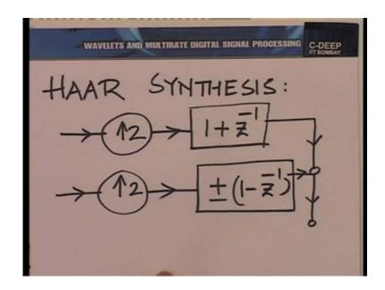
Now, there are several things to which we must pay attention. One is if you look at the structure of the analysis in the synthesis filter banks, the filters are almost identical. These are the two filters for the analysis side and these are the two filters for the synthesis side.
