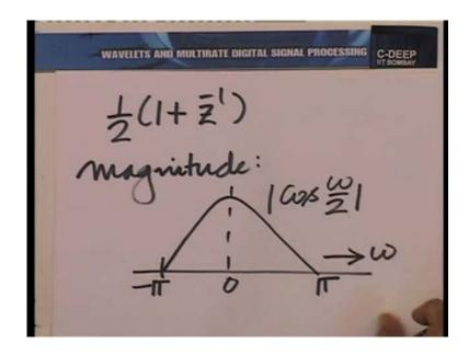
So, the situation is for the filter half 1 plus Z inverse. The overall magnitude response should look like this between minus pi and pi, I mean essentially, mod cos omega by 2 and the phase.
