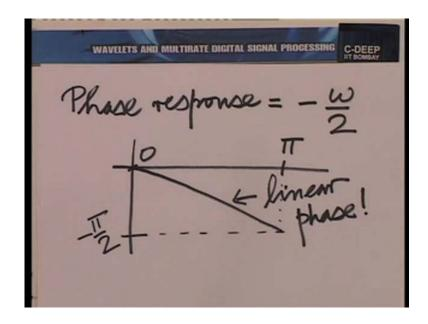
The phase response as we noted was minus omega by 2, so in the region from 0 to pi. At pi it would of course take on the value of minus pi by 2 and this is a straight line. So, in fact you get what is called linear phase. Now, linear phase is something very attractive in discrete time signal processing. In fact, one of the reasons why people go to discrete time signal processing from analog signal processing is because you can get linear phase.
