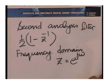
The second analysis filter and that is of course, 1 minus Z inverse into half. Let us again find out how the filter looks in the frequency domain. The frequency domain would show it as Z equal to e raise the power j omega where upon we have 1 minus e raise the power minus j omega by 2 and we play the same trick.
