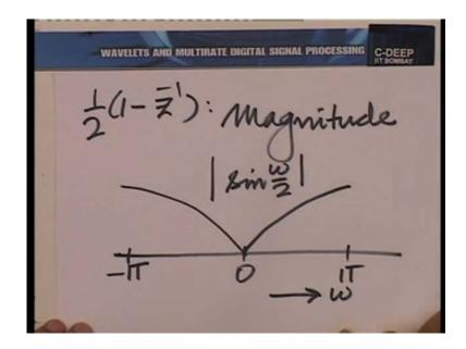
For the second filter, the overall magnitude response looks like this. Essentially, a sine mod sine omega by 2 and the phase response looks like this. Starts at pi by 2 there and goes to 0. It is a straight line segment, here it would start now. That is interesting.
