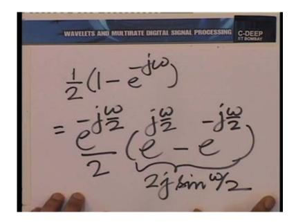
We take e rise the power minus j omega by 2 common and we have e rise the power j omega by 2 minus e rise the power minus j omega by 2 and once again, one can recognise this is essentially 2 j times sine omega by 2.
