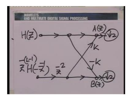
Z raised to the power minus L minus 1, H minus Z inverse, there, a Z raised to the power minus 2 here, a K there, a minus K there and the down samplers back again here. And we need to analyze the A Z created here and the B Z created here, which is now very easy to do, because I can write A Z in terms of these 2 and I can write B Z in terms of these 2. Let me do that.
