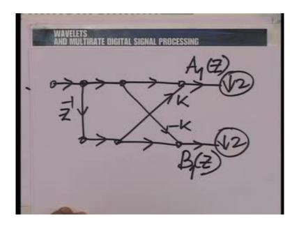
Well, the basis steps needs to begin from here, down sample there and then the lattice here, K times there, minus K times here, a summation here and we need to jump these down samplers here and study the relationship between these. So, we need to look at the following structures.
