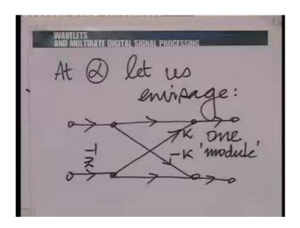
So, what I am saying is the following. If I add to this module, a delay prior to that, so as to increase the order. A delay here, which actually comes after the down samplers, is equivalent to a delay of 2 units before the down samplers.
