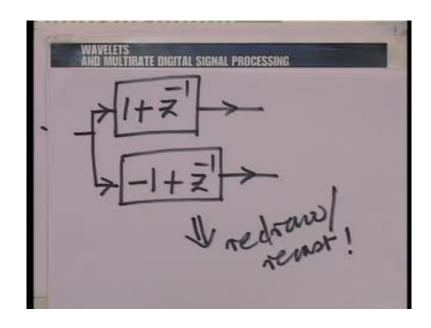
Now, in this case, let us rewrite the 2 analysis filters in such a way, that we have operations that are interchangeable, with down samplers. So, to do that, let us look at this structure carefully once again. Let us look at the pair of filters here. 1 plus Z inverse, minus 1 plus Z inverse. You know, the Z inverse operation is common. So, we can rewrite this, or redraw this, recast this, as follows.
