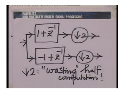
The corresponding high pass filter would be Z inverse H low minus Z inverse. And that is easily seen to be, Z inverse 1 minus Z, which is minus 1 plus Z inverse. And therefore, all in all, we have the following structure for the Haar analysis side.
