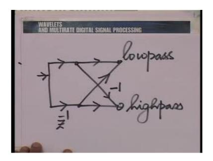
We could first have 2 branches, one on which we pass the signal as it is and the other, where we pass the signal delayed by 1. Now, we add these 2, to get the upper filter. So, this gives us the low pass branch. And we subtract these 2, use a minus 1 here, to get the high pass operation.
