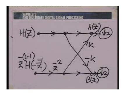
So, I have, A Z is very clearly, H Z plus K times Z raised to the minus 2 times Z raised to the power minus L minus 1 H minus Z inverse. And B Z is very clearly, in fact, let me just put back the figure before you to explain this. I am saying A Z is H Z plus K times Z to the power minus 2 into Z to the power minus L minus 1, H of minus Z inverse. So, H of this multiplied by Z raised to the power minus 2 multiplied by K and added here.
