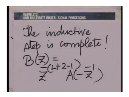
The inductive step is complete. B Z is Z raised to the power minus L plus 2 minus 1 A minus Z inverse. So, what we are saying is, the effect is that, the conjugate quadrature relation that we require on the analysis side is replicated one module later. So, each time we put a module like this, we at least replicate the relationship between the low and high pass filter in a conjugate quadrature structure analysis side. Now, for the basis step. That is easy.
