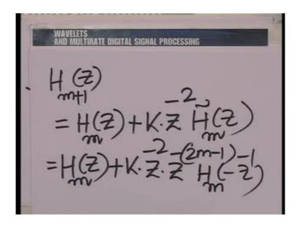
So, h 0 times K is the coefficient of the highest power of Z inverse in H m plus 1 Z. Let me put this back before you. What I am saying is, in H m plus 1 Z, K can only come with a highest power of Z inverse from here. So, therefore, we have now a mechanism to obtain K.
