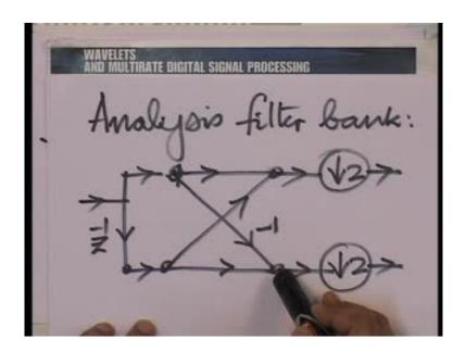
Now, once we have done this, we are in a position to put back the down sampler and the up and the down sampler for the moment. So, overall the analysis structure is like this. Let us put the Z inverse here. We have, followed by 2 down samplers and now, it is obvious, what we can do.
