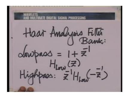
So, let us go straight down to putting down the Haar analysis filter bank. Now, on the analysis side, in the Haar, the low pass filter is essentially 1 plus Z inverse and we shall refer to this as H 1 Z or H low Z, let us say.
