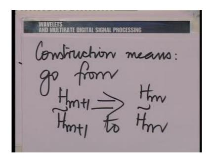
So, H m plus 1 tilde Z, which we assume is available to us, is equal to minus K times H m Z plus Z raised to the power minus 2 Z raised to the power minus 2 m minus 1 H m
