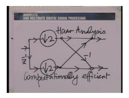
Let us draw the structure with that change. So, essentially the, the main theme here is, the down samplers can jump across adders, constant multipliers and branching. And doing that, we have a down sampler here, a down sampler there, an adder there, a minus 1 there and an adder there and this now becomes a computationally efficient structure for the Haar analysis side.
