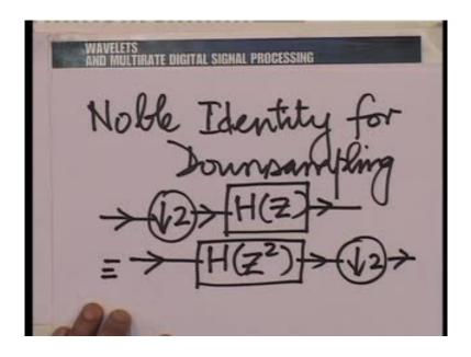
Now, what we are going to do is to use this principle of transposition to arrive at the noble identity for up sampling and of course, then we can prove it. So, let us put down the noble identity for the down sampling once again. Essentially, it says down sample
