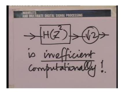
Whereas, this structure is the efficient version of this inefficient structure we should make a note of that. That is the a very important conclusion give we have drawn this structure is efficient computationally that is because we are doing away with samples that do not figure in the computational and this structure is inefficient computationally.
