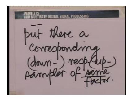
It means, first reverse the direction of signal flow; second, when reversing an up respectively down sampler, I will give a little bit of the caution has to be used, put there a corresponding down or respectively up sampler of the sampler of the same factor; that is, important same factor.
