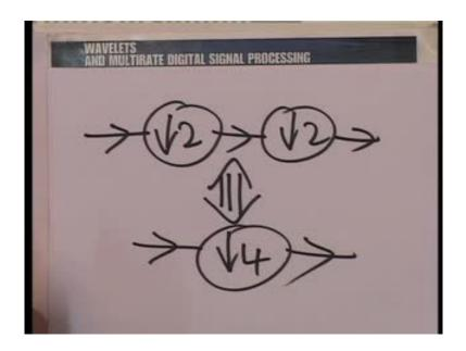
So, what we are saying in effective is down sample by 2 followed by down sample by 2 is equivalent to down sample by 4 and therefore, we have 4 filters that come of out of the this process.
