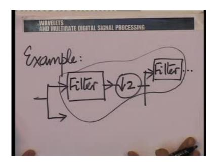
let us take an example. An example could be something like this: what happens in the discrete wavelet transformation? So, you have the filter followed by a down sampler again, followed by a filter in a down sampler and so on.
