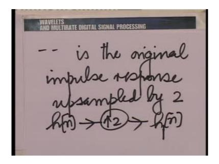
So, h n now this is what is called the noble identity for down sampling. In other words, whenever you have a filter transfer function where the oat odd samples of the impulse response are 0. The even samples could be non-zero; we could replace that filter followed by a down sampler by an equivalent operation where there is a down sampling first and then a filtering operation.
