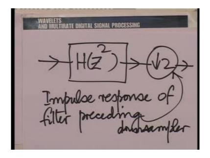
On the other hand, what you are doing in this structure here is first filtering that means, for example, before down sampling you are going to generate many samples here which are ultimately just going to be thrown away. To generate samples at this point you are going to do a lot of work because, you are going to do convolution operation here so this is an inefficient structure.
