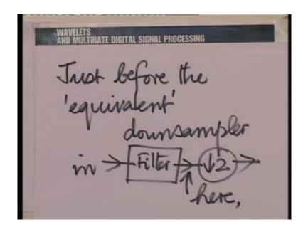
In other words, just before the equivalent down sampler, in filter and down sampler. So, at this point we have summation 1 going from minus to plus infinity h 1 x n minus 1 n minus 21. Now, it is very clear what the filter should be you know this is almost like a convolution; except that it appears as if you are taking only the even points in the impulse response.
