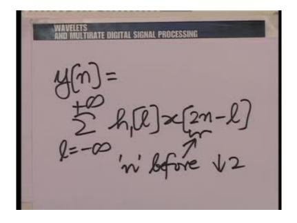
In that case, what we have here then is that y n is simply summation 1 going from minus to plus infinity h 1 1 x 2n minus 1. Once again, before the down sampler this is n so it is very clear what is happing here. The filter that operates before the down sampler is essentially 1 with the impulse response h 1.
