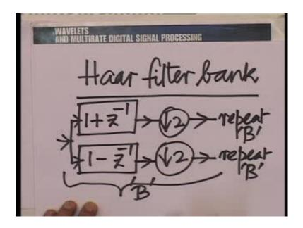
We have 1 plus Z inverse, forget about the factors of half inverse and so on. Let us just focus on the basic filter system function 1 plus Z inverse and 1 minus Z inverse. This is the analysis filter bank for the haar. Now, hold this whole thing in the bank B and what we do in the wave packet transform in haar would be to repeat B here and repeat B there.
