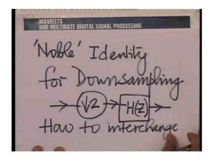
So, it is this kind of cascade that we wish to be able to address and therefore, let us consider the noble identity for the down sampling first. Now, the noble identity for down sampling emerges from the following consideration: how can we represent a down sampler followed by a filter? Let us call that filter H of Z; so we describe the system
