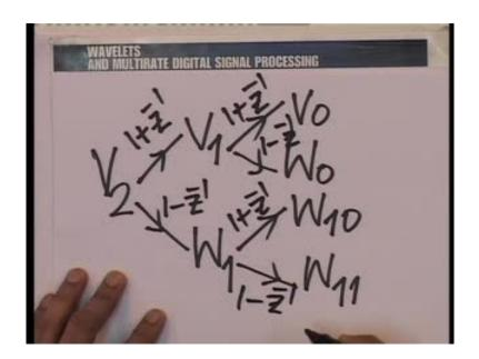
Correspondingly, if you go back to the structures here you realize that to come from V 2 to W 0 you should do 1 plus Z inverse and then followed by a 1 minus Z to the power minus 2 and to go from V 2 to W 1 0 you should do a 1 minus Z inverse followed by a 1 plus Z raised to the power minus 2. And, to go from V 2 to W 1 1 you must do a 1 minus Z inverse followed by a 1 minus Z raised to the power minus 2; so let us do these and complete the job.
