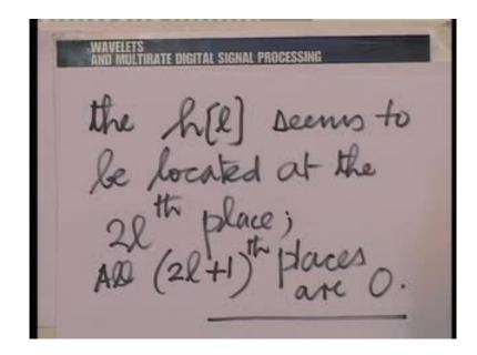
So, you are allowing only the even points in the impulse response to operate and the odd points have been analyzed this looks like a convolution but the h l seems to be located at the 2l th point.
