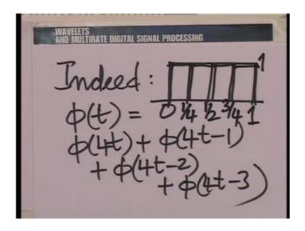
In fact, this sequence tells us how to expand an element of the basis here in terms of the basis here and as you can see this corresponds to the sequence 1 1 1 1 at the points 0 1 2 and 3. So, we are saying the sequence 1 1 1 1 expands phi t a typical basis element in V 0 in terms of phi 4t minus k phi 4t n and it translates you know, when you go from four V 0 to V 2 when you are going to dilate by a factor of 4; as what is meant by a down sampling by 4 and indeed, it is quite clear indeed.
