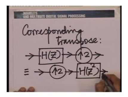
This is the transpose of this (Refer Slide Time: 32:17); up sample by 2 and the other way and then H Z squared and this is essentially, the noble identity for up sampling. So, what is the noble identity for up sampling? Say that if you filter followed by an up sampling by 2, it is the same thing as up sampling by 2 and then filtering by a filter whose impulse response is the up sample version of the impulse response of this filter. Of course, in both cases there is an up sampling involved.
