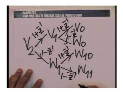
In other words, what we are saying is, when we consider this movement from V 2, you know what we are doing. If you remember, in the unless analysis process is to decompose V 2 into V 1 and W 1 and then followed by a decomposition of V 1 into V 0 and W 0.
