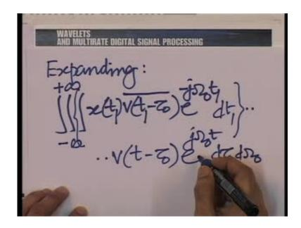
So, expanding we have a triple integral, one should not be frightened of the triple integral it just requires a little bit of rearrangement afterwards; so, the inner most integral is essentially to calculate the STFT and keep in mind, that we have a toutside, we should give a different name to this variable of integration here.
