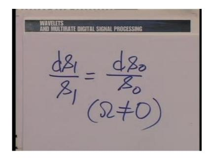
So, d s 1 by s 1 is d s naught by s naught, of course, assuming omega is not equal to 0, the only catch is that when omega is positive the limits are 0 to plus infinity, when omega is negative the limits are 0 to minus infinity and if we take care of that little detail, we have done away with the dependence on omega naught.
