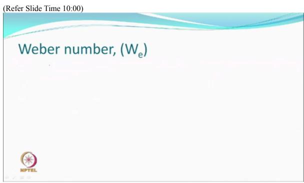
So this Weber number, it characterizes the atomizing quality of the spray and therefore the size of the droplet. It's a dimensionless number. So the units are chosen of all these in such a manner that you just get a number. So, roughly speaking, it's a ratio between the inertial forces and stabilizing forces, which are cohesive forces, like the surface tension itself. If surface tension is high, then it is difficult to separate. Right?
