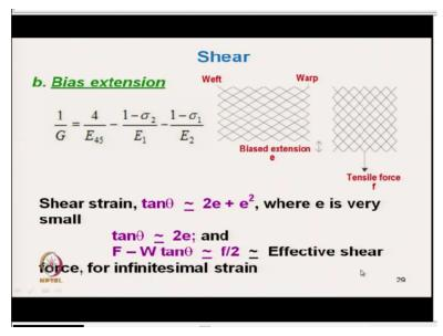
And the shear strain tan theta is related in the fashion like 2e+esquare where e is the biased extension by the force T. If we apply T force and then will have the biased extension, so that is tan theta we can measure. So, where it is a (()) (19:16) it is very small ok infinitesimal strain. So, that is e is very small if we take the e as a very small value this e square will be small, so that e square we can actually eliminate.
