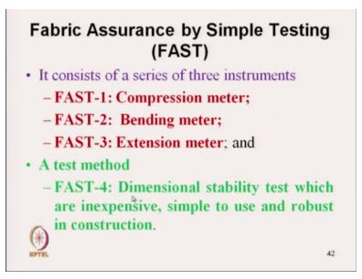
And there are basically 3 series of 3 instruments and 1 test method, so instrument FAST 1 is the compression meter which measures the compressional characteristics of fabric. Second one is the bending characteristics of fabric bending meter which actually works in the same principle of the Shirley instrument we have expressed we have explained here. FAST 3 measures the tensile and shear characteristics ok.
