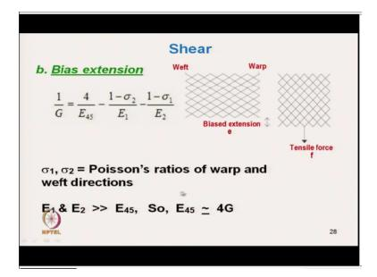
So, this is the equation, so E45 is almost equal to 4G ok. So, the sigma1, sigma 2 are Poisson's ratio. And here we can calculate the young shear's modulus of the fabric.
