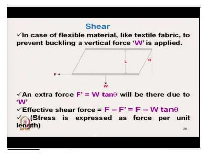
Before shear due to its high flexibility this fabric will buckle, this buckling will take place, so that buckling just to avoid this buckling prevent this buckling 1 vertical force is added applied extra vertical force W is applied. So, that the widthwise there is no buckling this becomes straight, so that extra force we have to apply in addition to F we have to apply an extra force just to have the W thus to actual balance the W.
