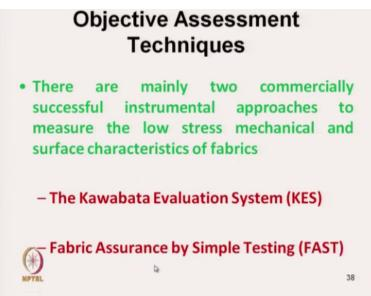
And in addition to this there are standard techniques the total systems of measurement of objective assessment of fabric handle. So, there are 2 instruments set of instruments are available commercially available ok and this those instruments the set of instrument measures the low stress mechanical and surface characteristics of fabrics, these are the Kawabata evaluation system for fabrics another is that fabric assurance by simple testing.
