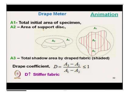
Now the measurement is done by using the drape meter where this is the a fabric ok fabric specimen without any with it is normal circular fabric space and A1 is the total area of the specimen we have cut the fabric and as it is flexible. Once we are placing the fabric with on a support disc of a certain known area A2. Then what will happen on it is own mass the fabric will start hanging.
