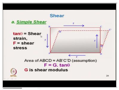
And where we can measure the angle of deformation theta and tan theta is shear strain and F is shear stress. Here assumption is that the initial that area of rectangular shape ok material the after
