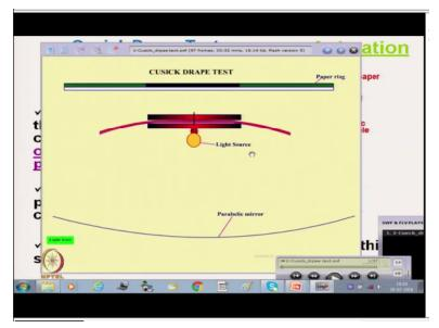
Now the light is actually falling the fabric sample specimen is just behind the light. It is not direct light is falling now it is now getting reflected and parallel light is getting reflected ok.
