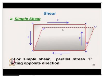
Now, so this is the simple shear, for simple shear parallel stress F is actually acting of in opposite direction that may this may be horizontal direction or may be vertical direction.
