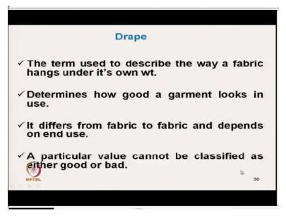
And drape the term is used to describe the way a fabric hangs under it is own weight. So, if we actually if we hang the fabric this fabric under it is own weight, how the fabric will get actually will hang will make some profile. That shows the drape characteristics and it determines how good a garment will look like. So, it is not only the garment for any other fabric like our cottons or any other fabric which actually requires a fall.
