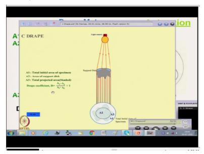
And we are calculating the drape coefficient now main problem with this system is that the light which is actually diverging. And actual area whatever we are getting it is not the actual area of the fabric projected area it has been actually enlarge this area is enlarge. So, that is why the sometime this keeps error value depending on the length of a distance from the light source ok. And what we can do to eliminate this problem we can have 1 system where light is not diverging time.
