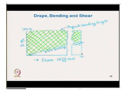
And last part is that there direct relationship diagram shows the relationship between shear stiffness, drape coefficient, drape % and the bending length. Now try to see one by one suppose a fabric is having zero shear stiffness. This is the zero shear stiffness ok, at zero shear stiffness if the fabric bending length that is bending length means it is highly flexible and the imaginary there is a zero shear stiffness there is a in that case the drape coefficient will be zero.
