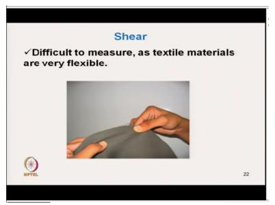
So, it is difficult to measure, so shear characteristics it is very difficult to measure. Because it is flexible, for any sheet material shear characteristics measurement it is not that difficult ok. It is basically when suppose there is a material any other material stiff material. And we are gripping in this is the 1 grip point ok. The material we are gripping now we will apply 1 force, so with this which is parallel to the base ok.
