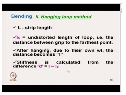
And L is the length of strip, L0 we have discussed it is undistorted length of loop that is distance between grip and the farthest point. And after hanging on it is own weight the distance there will be some distortion. And the distance becomes 1, 1 is more than 10 and the deflection that is the stiffness is calculated based on the difference d is 1-10, so we have discussed.
