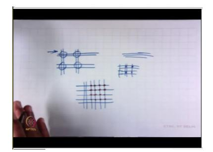
We have made a fabric with say rods highly polished extremely polished rods we are placed OK and this there is no friction there is a zero friction, zero friction between the rods. In that situation imaginary if we apply force, so there will be no shear stress, so that will this will simply slight there is no shear stiffness. But as the rods there are rod we can see we can assume the rods are highly stiff that means there is a infinite stiffness that means it will never bend ok.
