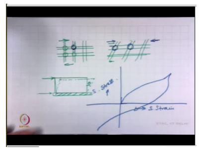
Suppose these are the warp yarn ok, so weft yarn and these are warp yarn. Now when we deform when we apply force ok this yarns will get deform very easily there will be because there is no actually positive binding. So, they will deform easily due to its inherence fracture, now if it is asked instead of textile material instead of say woven fabric or knitted fabric. We use any polythene sheet, so for any polythene sheet the we can incorporate any characteristics.
