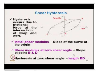
Now what is shear hysteresis?. Now shear hysteresis is that say suppose this is a fabric initial stage. Here at the initial stage although there is no from positive binding. But the fabric to yarn to yarn the warp yarn to weft yarn, this yarn to yarn friction will be there ok. This the shear force when it is actually deform there will be frictional sliding. That means suppose this is the force and what we are doing we are trying to deform ok.
