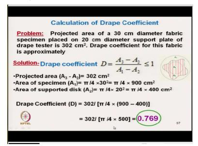
So, the problem here to calculate drape coefficient is that projected area of **3** 30 centimeter diameter fabric specimen placed on 20 centimeter support plate of drape tester is 302 centimeter square. Drape coefficient of fabric what will be the drape coefficient that means what is the projected area, projected area is means the shadow area-the area of the support disc that is the projected area.
