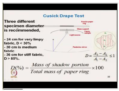
And 3 different specimen diameters is recommended ok when the fabric drape coefficient is very small. So, less than 30% 24 centimeter for very limpy fabric ok, for medium fabric is 30 centimeter and for stiffer fabric 36 centimeter. So, these are the various fabric sample diameters are given and then the drape coefficient we can measure ok.
