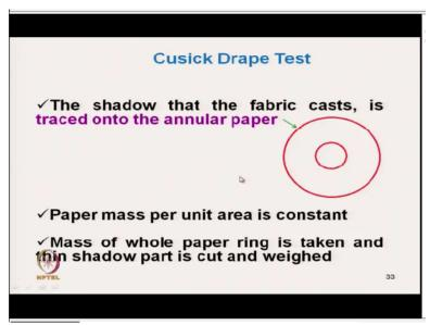
And that it is done by the Cusick drape tester ok Cusick drape tester is that the shadow that the fabric cost is traced on a annular paper where this is an annular paper. And the shadow we actually whatever it is casting it is that shadow we are just cutting out. Now this in this annular ring this is paper of known mass per unit area. So, mass per unit area of the paper is constant and this inner it is a whole this is the size of the support disc.
