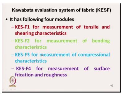
And there are 4 modules in Kawabata system KESF 1 or FB 1 for measurement of tensile and shear characteristics. The module 2 for measuring the bending characteristics module 3 measures the compressional characteristics and module 4 which measures the surface roughness and friction characteristics, so this 4 modules are there.
