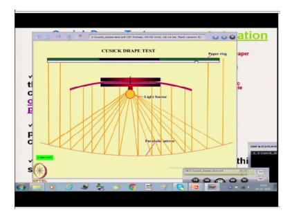
Now as the light beams are exactly parallel, so that there is no divergent the shadow we are getting here we are tracing here which is exact shadow of the fabric. And we take the difference ratio of the mass we will get the drape coefficient and expressed. And we can express in terms of factor also or we can express in terms of % by multiplying by 100.
