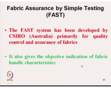
And similarly the FAST fabric assurance by simple testing which is developed by the CSIRO Australia and there the it gives the objective indication of fabric handle characteristics.
