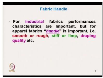
Now fabric handle if we see so far industrial fabrics performance characteristics are important ok, their performance characteristics means their tensile strength, abrasion strength. So this type of characteristics are important ok, their permeability ok. But for apparel fabric along with other characteristics the handle is extremely important which actually handle as you takes care of smoothness, roughness which is a surface friction type characteristic.
