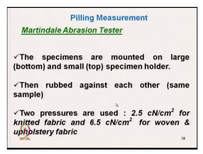
Another method is that it is Martindale abrasion tester where the specimens are mounted on a large bottom and small top specimen holder. Here the thing is that in Martindale abrasion tester where we use 1 abradent standard abradent sample in the bottom normally ok. But here in that small modification is there here the both bottom and top specimen holder the same fabrics are tested, so same fabric specimens are tested and they are actually rubbed against each other.
