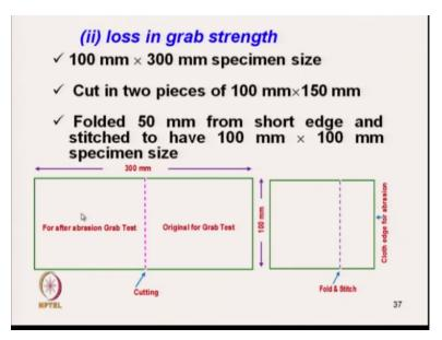
And next method is loss in grab strength where the specimen 100 millimeter/300 millimeter specimen is actually it is cut 10 centimeter/30 centimeter this is the 30 centimeter/10 centimeter, this is a specimen. Now we cut this fabric into 2 equal parts, so that means the specimens are it is a 150/100, so specimen size becomes 100 millimeter/150 millimeter. Now we keep 1 specimen as standard specimen ok this is the standard specimen we keep separately.
