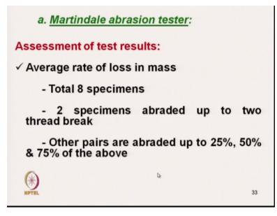
Now assessment of test result normally in Martindale abrasion tester we measure the loss in mass say in milligram/1000 cycle. So, how do we measure, so where what we do total 8 specimens are taken, 2 specimens are abraded up to 2 thread breakage, that is the extreme end point ok. So, that we know that and we note down the number ok we note down the number of the cycles required other pairs are abraded 25%, 50% and 75% of the above means.
