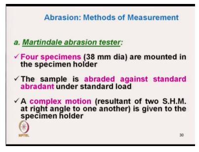
Now the methods are there are several methods one is the Martindale abrasion tester where 4 specimens of 38 millimeter diameter are mounted on specimen holder and the sample is abraded against standard abradant under standard load. And a complex motion is given, so which is actually of 2 simple harmonic motion at right angle. That type of motion is given to the specimen holder.
