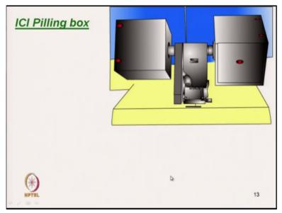
And these are placed on this ICI pilling box where all 4 samples are taken the tumbled together in a cork lined box ok this is a cork lined box and allowed for certain revolution of time. So, it is actually takes certain number of revolution, so that is how this instrument goes. So, we can allow it to rotate for certain time.
