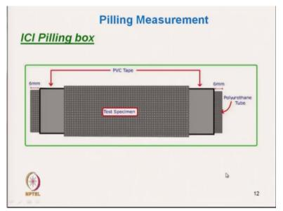
Like this, this is a fabric sample and here is a PVC tape and this type of the loose ends are actually sealed with a PVC tape.
