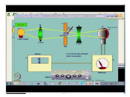
So, we can see here by this animation, so light is moving through and it is without any material. So, this is there is no material it is there now it is material is there material is flowing that is moving ok yarn is moving. And then light is falling on it ok photoelectric sensor will sense the amount of light which is proportional to the diameter of the yarn as yarn moves the diameter varies at different location depend position.
