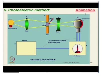
Here this is the light source lens arrangement is there this is the slot is there at yarn is passing through this. And depending on the diameter of the yarn the light will pass through this and it is in photoelectric cell. This will detect the amount of light which is proportional to the diameter of yarn and as the yarn moves this will record the variation in diameter.
