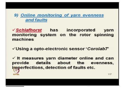
So, after that we will just try to finish quickly, so we can also measure the evenness or faults online. So, whatever things we have discuss or basically this were actually the offline techniques. We have to take the yarn or material from the machine and test offline. But there are techniques like in Schlafhorst the Corolab that rotor spinning machines there. They have fitted the optical sensor with each and every end each and every rotor actually rotor box ok.
