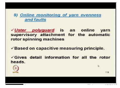
Uster polyguard also they are which works on the capacitance principle and it keeps the information on variability. So, with this we have to come to the end of the session evenness ok. In next session we will discuss the other parameters, other parameters means we have completed the **f** fibre we have completed fabric yarn. And now we will see test methods, testing techniques or fabric ok till then good by thank you.
