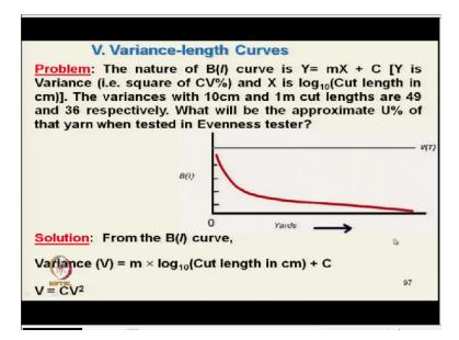
The nature of B(l) curve is given it is a logarithmic curve ok. So, which is mX+C where Y is in Y is the variance square of C%. And X is the log of cut length now here although this is the shape of the curve now we can form curve where Y-axis is in log. If we have the logarithmic value then the curve will be typically it is a straight line curve. So, many manufacturer they have programmed it is a in the logarithmic curve not in this form.
