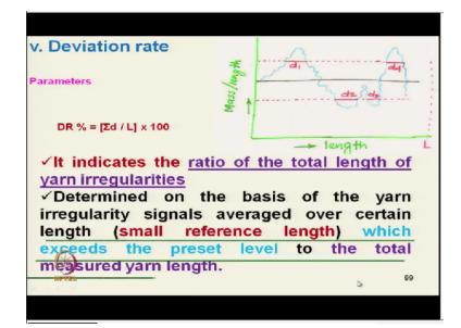
Another way of expression of variability is called deviation rate, deviation rate is nothing but it indicates the ration of the total length of yarn irregularities this is the definition. It is a ratio of total length of yarn irregularity that means this is the yarn irregularity plot ok mass/length. Now here we have certain reference length like what we tell? The DR% of 50% and more, so this is the yarn, so this is the mass/unit length which is 50% or more than the mean mass/unit length.
