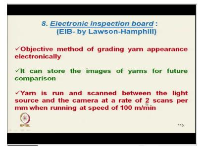
So, another instrument which is electronic inspection board, so where it sense in Lawson-Hamphill instrument, where it actually works in photoelectric principle. And objective method of grading yarn appearance it stores the data yarn diameter data and automatically form the yarn board without as we have seen yarn board rapping. It will automatically form the yarn board and it will compare with the standard.
