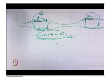
Now physically if we see suppose this is the mass mean+- +50% and above. This length is mean +- +50% and above, so this length is actually measured this is d1. Another portion here this length d2 this length is having mass+50%, in this way we will keep on adding d1+d2+d3 only those lens portion of yarn length of those portions of yarn where the mass/unit length more than 50%.
