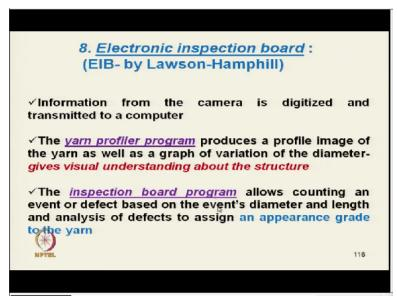
So, information from the camera is digitized and transmitted to the computer. Yarn profile program produces a profile image of the yarn as well as the graph of variation of the diameter. So, this profile program is there and inspection board program is there the 2 types of program one can have, so automatically it will form yarn board. And it will automatically be credit yarn appearance one, so you do not have to do anything with the standard grid.
