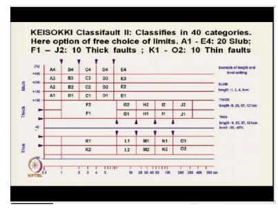
So, it is simply the software we can keep on adding the variability ok different labels. The basic principle is same.
