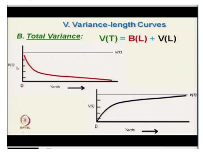
So, BL curve and as the yarn cut length increases the between length reduces, on the other hand as the cut length increases the variance within length increases. So, effectively the total variance is the summation of between length and within length ok. Now we will see one practical numerical the problem is here.
