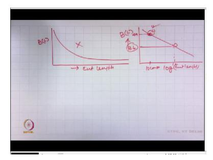
It is very practical problem here now we know that this is the BL curve it is a length cut length but if we take the cut length in logarithmic form normally we get the printout in the logarithmic form. And BL, so this curve will be like this ok this is the curve and the in the instrument they give this type of print not this type of print out. This is the print out now looking at this here the problem is that at certain cut length.
