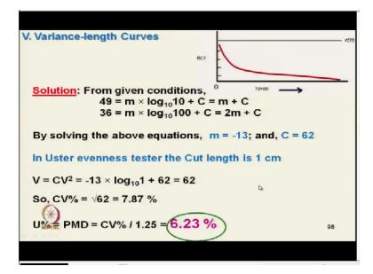
From given conditions the 49 is the variance m with the cut length of 10 centimeter+C the m+C log10 is one m+C equal to 49. And for 1 meter cut length 1 meter means 100 centimeter 36 m log100+C equal to 2m+C, from this 2 equations we can measure the we can get the value m and C. So, by solving this equation m equal to -13 and C is 62. Now problem is that we have to see the evenness tester as we have already mentioned in last class.
