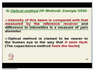
So, intensity of this beam is compared with that measured by the reference receiver and difference in intensity is measured it is a measure of yarn diameter ok. And that the optical method is claim to be nearer to human eye in the way it sees the fault ok. And capacitance
