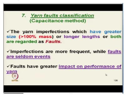
Next is that the yarn fault classification, although the principle is same as that we have seen the are capacitance type of method. But here we do not measure the thick thin or neps, thick, thin, neps are actually inherent nature inherent characteristics of yarn. This thick, thin, neps we cannot eliminate we cannot take out from the yarn because they those are very frequently occurring. We cannot we can only try to minimize those ones.
