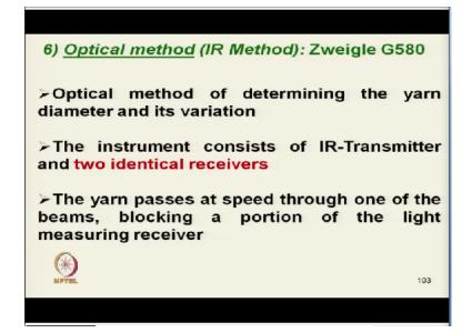
Next is that another optical method which is infra red method Zweigle G580 model which is actually it is optical method of determining the yarn diameter and it is variation. And the instrument consist of 2 IR-transmitter of in identical in nature and identical receivers will be there and one of through one the ray ok. The yarn will pass it will be blocked partially and the it will be compared with the reference receptor.
