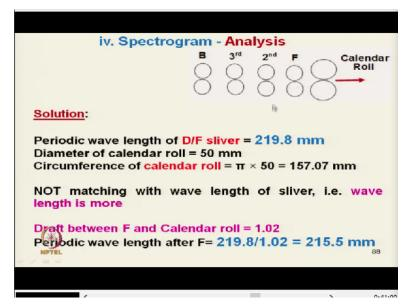
The periodic wave length of draw frame sliver is 219.8 millimeter and diameter of calendar roller as it is given it is a 50 millimeter. This calendar roller has got 50 millimeter suppose we assume the calendar is now defective. Now it has being now we are identified that the ring frame is not culprit the roving frame is not the culprit. The draw frame where it the periodicity has generated now we have to identify among all this rollers 1, 2, 3, 4, 5 sets of rollers which roller is problematic.
