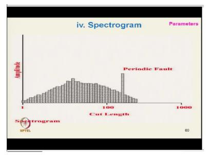
Now this is the periodic fault this is the normal cotton ok normal, for normal cotton yarn without any periodic fault it is there ok. And it does not show it is very clear it does not show any it is level of uniformity level of it never shows the level of uniformity. It shows only periodic fault and periodic it is important because we can actually the periodic fault as we have seen it creates measure problem in appearance.
