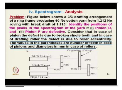
Now we will try to see few practical problems and what is the implication of how to use the spectrogram? What is the use of spectrogram? Now figure here it shows 3 over 3 drafting system and it is producing 40 Ne cotton yarn from 1.211Ne roving with the break draft of 1.115. So, break draft here between back roller and middle roller 1.115 break draft identify the position of peak in the spectrogram.
