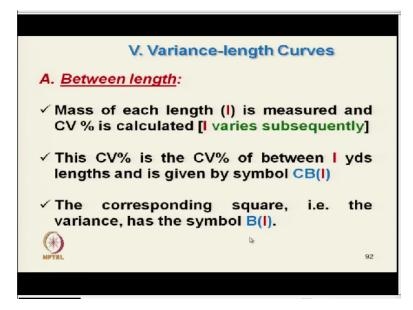
So, variance between length mass of each length 1 is measured and CV is calculated ok 1 varies subsequently. And then the CV is the CV between the 1 length and giving the CB(1) and if we take the square of that variance it is a B(1) curve ok.
