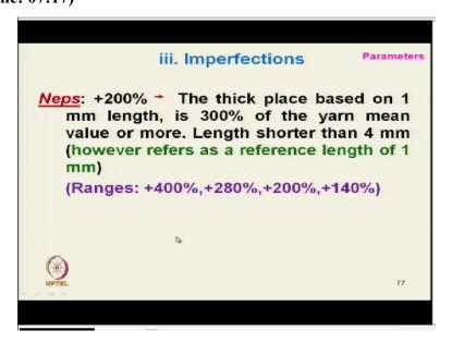
Neps+200% neps +200%neps means it is the total mass/unit length will be 300% of the mean value that one mass we will very careful like 280% neps means the mass/unit length is 380% ok that means +200 280%. And it is a reference length is 1 millimeter shorter length that is less than 4 millimeter. But it is actually specified as 1 millimeter length.
