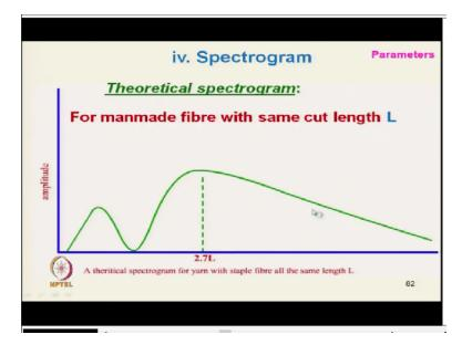
So, if we plot this will get this type of curve this is the if we simply plot this equation this is the type of curve and for manmade fibre where the length number of fibres and length of the fibres are fixed for constant length 10 fibre length will get this type of one. And this is the 2.51 which is actually shows the position of the drafting wavelength ok. But for cotton where the variability is there variability in the fibre length is there.
