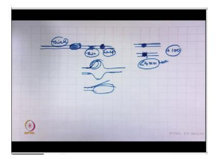
So, that it is due to the problem in the technology ok problem in machine ok the we cannot have yarn staple yarn without any imperfection, only thing we can reduce the intensity reduce the number of imperfection. There will be definitely some thick places, thin places or names, so thick places there will be little bit more number of fibres and average. There will be number of less number of fibres in the cross-section than average or there will be some node type.
