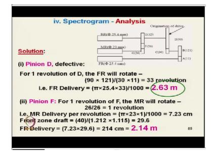
This is the situation now first condition is that the pinion D is defective. So, this is the pinion D now let us see the pinion D is rotating it is driven. So, once and it is got one defect when one teeth actually broken, here as it is driver, so this will give drive to the back roller and middle roller. But this teeth will not affect broken teeth will not affect the motion of the back roller and middle roller. Because they are rotating ok they are basically it is getting drive.
