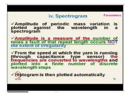
Now coming to one of the most important diagram or most important actually method of measuring the technique of measure in the periodic fault the spectrogram. The spectrogram only talks about the periodic fault if the yarn if the material does not have any periodic fault. Then spectrogram will not show anything ok, so the amplitude of this periodic mass variation is plotted against the wave length in the spectrogram ok.
