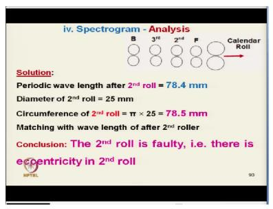
And if we see the circumference of second roller with the diameter of 25 millimeter it comes exactly same as 78.5 millimeter. It is matching with this value that means the fault is generated by the second bottom roller. This roller is defective ok matching with the wavelength after second roller and conclusion is that second roller is faulty that is there is eccentricity in second roller.
