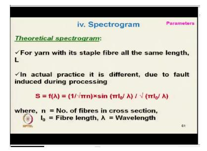
And this here this is the zone initial zone 2.5 to 3 inch zone. Here if it is there it is shows there is no such hump that means there is no problem of the this yarn with the wavelength drafting your problem is not there. But there is definitely there is a periodic fault is there at this wavelength, so what is the wavelength? If it is basically it is a 100 centimeter may be say 1.5 meter or 2 meter say logarithmic skills sometime.
