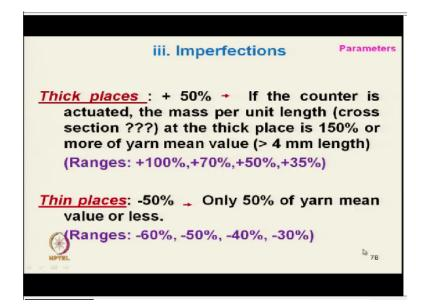
And the thick places example for say 50% thick place 50% level. So, what we calculate?, we calculate the number of thick places number of places where the mean value is +50% it is actually thick place thin places are expressed in terms of + or -, +50% means the mean value if we talk about the 100. And then + that means 150% that means 50% more than mean, if the counter is actuated the mass/unit length that is cross it is proportional to cross section.
