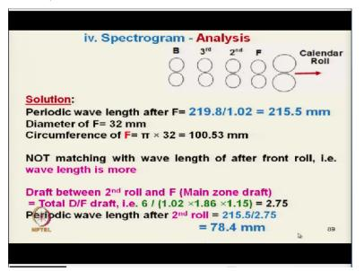
So, wavelength of the after front roller is 215 millimeter and diameter of front roller is given it is a 32 millimeter diameter is given. And then circumference of front roller we can calculates 100.53 ok still the wavelength is more than the circumference of that front roller F. So, that means front roller is not actually generating the fault, so not matching with the wavelength after front roller that is wavelength is more.
