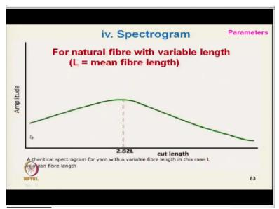
The typical curve is like this, this is for natural fibre like cotton we have this type of length. And here this is if at this point we get the this is due to the variation of that periodic variation of the drafting wave. So, 2.5 to 3 ok 2.82 length this is the at where automatically it will give the highest hump ok.
