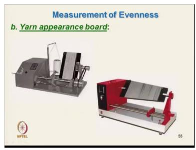
Now this is the typical yarn appearance board wind up this is board read of basically 2 types 1 is the rectangular, another is trapigenic. So, this I this way, so we can simply wind the yarn ok this
