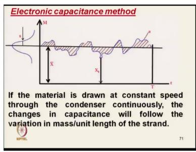
Now try to see here if the material is drawn at constant speed through the condenser continuously the change in capacitance will follow the variation of mass/unit length. So, it is capacitance change it is actually it is exactly it will follow the mass/unit length variation.
