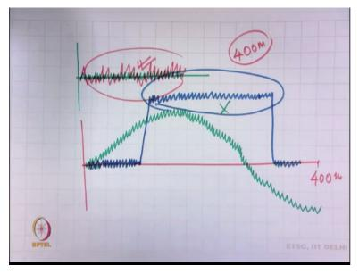
Now this is the this is 1 diagram ok now another yarn is having diagram like this from this looking at this diagram we can make out which one is more clearly we can see that this yarn rate it gives poorer actually evenness ok. This yarn green it is even, so similarly in this picture this diagram ok diagram this one it is even here although there is a variation it is even. But this yarn 2 this one bottom it gives very high variation, it is not that even ok.
