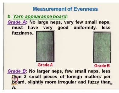
Now, so grad A means best quality portion ok that means depending it does not depend on the count ok, it is basically overall grading. So, in that case there is no large names very few small names ok, no large names because few why few small names because we are talking about the say this is basically for cotton yarn there will be some names short fibres will be there, there will be some neps.
