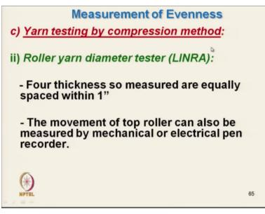
Another measurement is the by using compression it is the yarn diameter actually tester roller yarn diameter tester it is a simple tester where.
