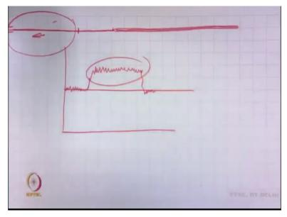
Now the thing is that suppose there is a yarn initially it is a thin yarn and after that it has got say actually yarn, thin by some mistake ok initial portion thin yarn. Now if we place if we test this yarn in say uster machine or any evenness tester suppose this yarn is moving like this in the capacitance tester it is moving. So, within the initial length it has actually gets the mean value, so this has been plotted.
