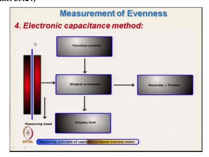
Now this is the principle here it is the measuring head and here the length is 1 centimeter as I have mentioned here and signal processing display you need, recording you need, printer everything is there.
