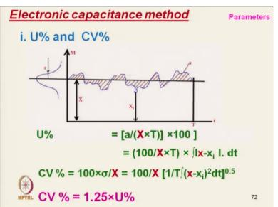
Now how to calculate the then U% from this curve, here this is the variation in mass/unit length as actually are you are getting the capacitance value only thing it is a factor of K. So, factor of K
