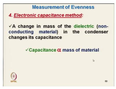
And then a change in mass of the dielectric ok change in mass of the dielectric material like in our case it is a yarn non conductive yarn material in the condenser changes it is a capacitor. So, capacitance is changing which is proportional to the mass of the material ok, so Km is there capacitance.
