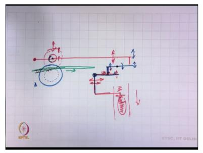
Here the roller which is motor driven ok and this is driven roller motor driven ok A and here it is a plunged top roller with a plunge. So, top roller I am drawing with a red color top roller and which is plunged ok and material, material moves through this in between this, this material is moving ok. And for this any unevenness this roller will move up and down but the in this instrument the arrangement is there we have to record this.
