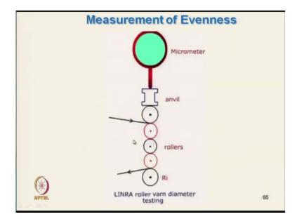
This is the yarn there are different rollers are there and yarn is moving on this depending on the diameter variation and this will move up and down. And this can be recorded by using micrometer or maybe by electronic arrangement we can directly measure this thickness variation. (Refer Slide Time: 26:40)
