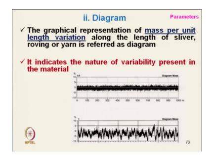
Now coming to one of the most important graph picture which gives the diagram, so the graphical representation of mass/unit length variation along the length of sliver, roving or yarn is reflected as diagram, it indicates the nature of variability present in the material.
