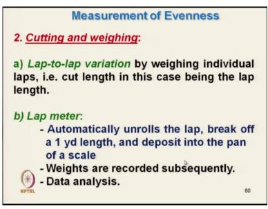
So, lap to lap variation, so what we take the mass of lap and then measure the take the whole lap and then measure the mean and CV% that is a lap to lap variation and lap meter is there where automatically 1 yard length is cut. And then measured the mass of that 1 meter and we can measure the CV% standard deviation, the words are recorded subsequently and data analysis is there.
