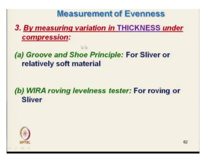
Next technique is by measuring the variation in thickness ok, so this material suppose this is sliver.
