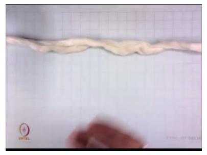
Here this sliver thickness that if we measure the thickness of the sliver at different portion that will give the idea indirect idea of mass variation. There are various techniques of measuring the thickness variation by measuring thickness variation we can measure the irregularity of material. So, one of them is that it is called groove and shoe principle this is actually used for sliver or relatively soft material where number of fibres in the cross section is large.
