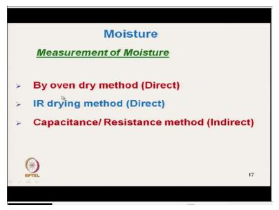
Now how to measure the moisture content, so moisture measurement it is very simple we actually follow 2 methods. One is that it is by oven dry method basically 2 methods we follow, one is directly take the material and then we dry the material in oven to make it bone dry, that is
