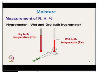
Now how to measure the relative humidity, as we have just discussed that the relative humidity is the measure of content of air ok, content of how much moisture present in the air that is are relative humidity. Now the basic way of measurement it is called dry bulb, wet bulb principle this is once simple thermometer, it is called dry bulb ok. This dry bulb thermometer it is placed in this room suppose it is a dry bulb, in that atmosphere it is kept.
