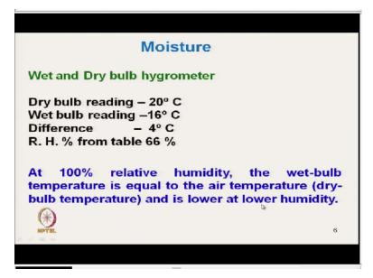
Now dry bulb reading suppose it is 20 degree Celsius, for example in certain condition and wet reading is 16 degree Celsius. So, we must take the difference the difference is 4 degree Celsius and from table there is a standard tables are level and from the table we can read that the relative humidity is 66%. So at 100% relative humidity as we have discussed the wet bulb temperature is equal to the air temperature.
