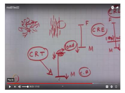
Let me draw here this is the fix jaw. Okay here it is this one is the moving jaw. And if this moving jaw moves at a constant rate that means elongation will be at constant rate. So this is will be a constant rate of elongation. Now next is that this fixed jaw. This is a moving jaw. Okay. This jaw is moving in such a fashion that loading on the yarn is at the same rate, loading on the yarn increases at the same rate. Okay. Suppose 1 kg per minute okay.
