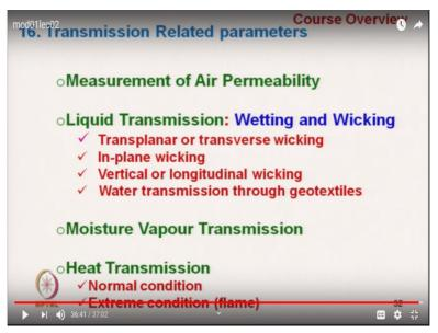
And next is that the transmission characteristics of textile material. A transmission characteristic starts with the air permeability. So basically any fluid transmission through material will discuss measurement of air permeability. We will discuss here then liquid transmission. So wetting and wicking. So absorption of liquid and transmission of liquid wicking characteristics we will discuss here.
