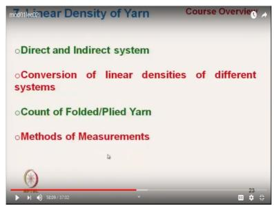
Next is that linear density of yarn. So, linear density means the mass per unit length or length per unit mass because there are two process one is a direct process of measurement, direct system which is expressed in terms of mass per unit length. And indirect system is that length unit mass. So, that this detail we will discuss and their interrelationship we will discuss. And
