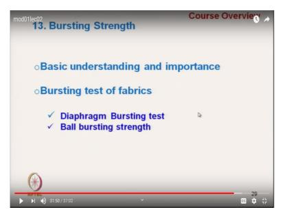
Busting is also not normally not common testing. It is for a specific application we test. And there are various technical textile where busting is extremely important. Like parachute fabric or filter fabric where we need to test busting. Normally we do not test busting for apparel fabric. But for technical fabric it is required. Busting like for geotextile busting system is important .Where the direction of force is not unidirectional.
