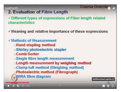
We will start with the evaluation of fibre length okay. Different types of expressions of fibre length and related characteristics. Like fibre length are expressed at with by a different terms, it is not the fibre length. We sometimes call it as mean length; we can call it as span length. Span length is also the divided into various terms 2.5% span length, 50% span length, okay. And this staple length, upper half-mean length, so for upper quartile length so various terms Okay.
