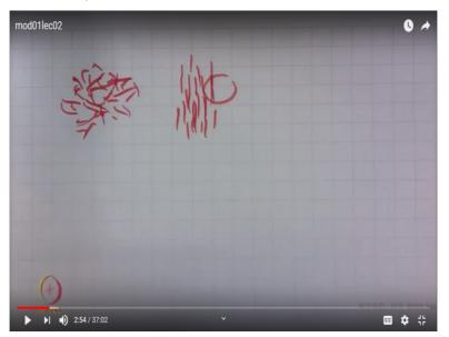
Suppose this is the tuft okay, where the fibres are randomly arranged okay randomly arranged. So we can pick up small quantity of tuft okay. There it represent entire quality entire because here we have short fibres, we have long fibres everything is there okay. But in sliver if we see this slivers are arranged in a particular order. Say parallelism here if we try to pick sliver from the side.
