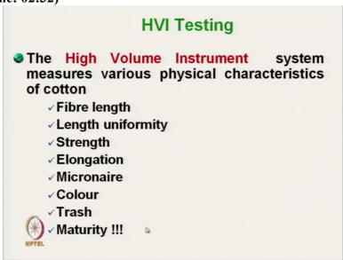
Now first we will discuss about the High Volume Instrument testing. This High Volume Instrument System measures various physical characteristics of cotton fibre. Last segment what we have discussed, like for measurement of fibre characteristics a particular technique used for a measurement of particular characteristics ok. But here in High Volume Instrument,
