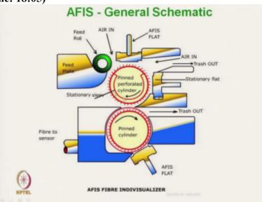
This is the basic schematic diagram, ok general schematic diagram; here the fibre is feed here ok. That is normal like carding we feed, this is the feed roller and feed plate, the fibre is feed here. And here it is the feed perforated cylinder, which actually opens the fibre, against the flat ok, AFIS flat. So, against this flat the fibre gets individualised. These are the stationery flats, ok. The individual flat, individual fibre, are carried away by the; this pinned cylinder.
