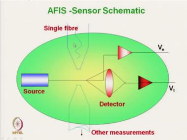
And this is the fibre sensor. From the sensor, single fibre is from that equipment, from the pinned cylinder, this single fibre is coming. Now here it is a source light. And it detects the total fibre characteristics. Fibre length, if we know the speed of flow, and time required to cross this line, then it is basically we can calculate the length. And the direction of flow in such a fashion, it, fibres will flow in a straight line.
