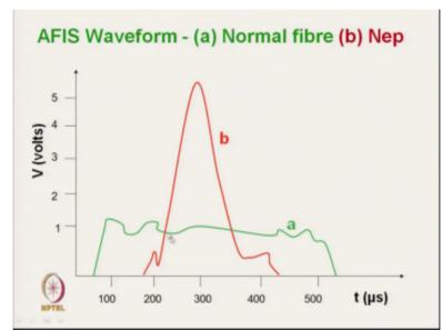
And we get the AFIS and this is the normal fibre ok this is the normal fibre that we have formed and if the fibre are in the nep form, we get this type of peak. So, we can get also in the AFIS the nep content ok, not the number of this type of peak gives the nep content ok and this is the, so we can easily separate out the normal fibre along with the nep. And also as it is the light principle here we can also calculate the diameter of nep.
