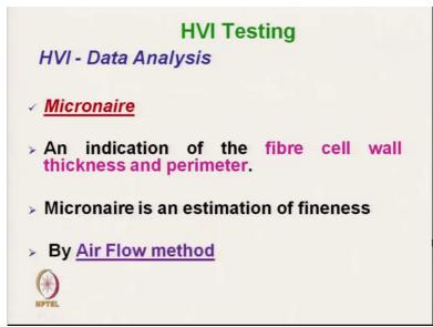
Then micronaire, an indicator of the fibre cell wall thickening and parameter ok. So, that is the micronaire value which is actually been indirectly it says that it indirectly measures the; that is maturity also. That is the why here only it measures the micronaire but it says that it indicates the maturity of fibre also. And micronaire and estimation of fibre fineness it follows the air flow method.
