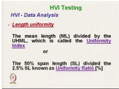
The Mean Length of fibre divided by the Upper Half Mean Length we get the Uniformity index or the Uniformity ratio we can measure this things are exactly same as the that we have discussed earlier. (Refer Slide Time: 05:54)
