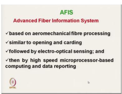
Now coming to the next, set of instrument which is AFIS, Advance Fibre Information System ok. This advance fibre information system is that, is the, it is based on aero mechanical fibre processing. What is aero mechanical fibre processing? It is just like a carding ok. We take the fibre mass and by, it is carding, it opens the fibre. It individualise the fibre. And then the individual fibre are transported trans means transported through a sensing device ok.
