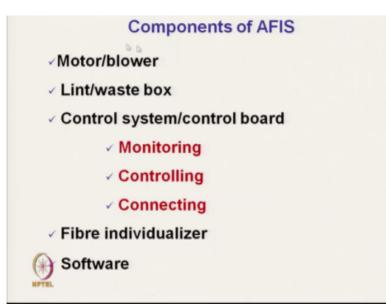
And the components are motor or blower, lint/waste box, control system/control board, it is monitor, monitoring, controlling and connecting. Then it is the Fibre individualiser. The fibre individualise the fibre. And we need software. These are the different components. **(Refer Slide Time: 18:05)**
