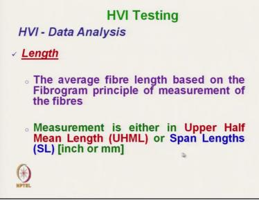
Now the length, the measurement technique we are not going to discuss here, because it is exactly same that we have discussed in fibrogram. Now length data that is the average fibre length based on the fibrogram principle of measurement of fibres ok, this is the same principle. Here also we measure the Upper Half Mean Length and Span Length. (Refer Slide Time: 05:31)
