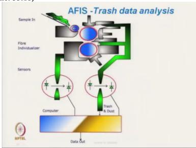
And this is the trash data analysis. So here the trash counter, trash and dust are coming. This is the; this sensor is for fibre. The two different sensors and trash is getting separated from
