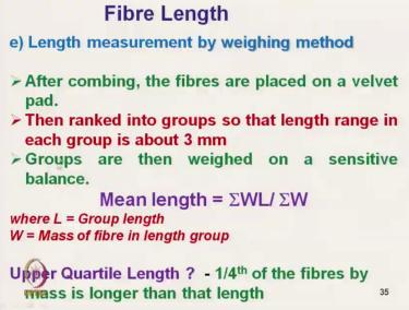
So, length measurement by the weighing method; this is actually done this is used in woollen industry and also in cotton Industry. So what it is done? After combing we can comb or we can we can do multiple drafting and drawing ok. Fibres are placed on velvet pad. Then what we will do be rank into groups so that the length range in each
