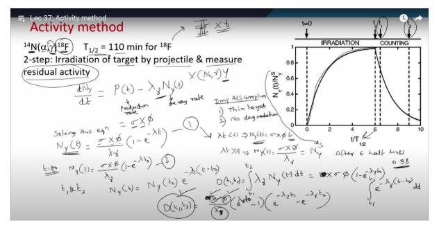
Now after irritation is stopped and kept in front of the detector now you have measured the gamma rays in between two timings like t 1 and t 2. So, how you can write down this equation for the number of nuclei this N y t is and now I am writing after t = t 0 the number of residual nuclei is undergoing a new decay so P of t is 0. When P of t is 0 only decay is happening how this time evaluation of residual nuclei is happening very simple.
