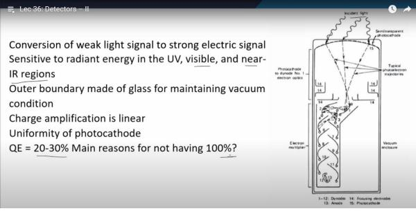
So, now this photomultiplier tube is basically conversion of optical photons into signal electrical signal. How it works? So, this incident light falls on the photo cathode and it converts into strong electric signal by multiplying the electrons. And here at the photocathode the conversion is taking place with the help of photoelectric effect and sensitive to radiant energy in UV, visible and near IR regions.
