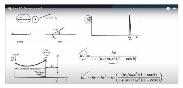
scattering and applying conservation of energy and momentum one can derive the energy of the scattered gamma and recoil electron.
