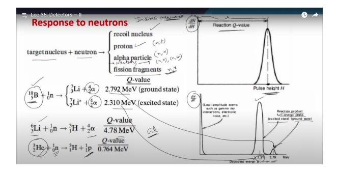
And the materials which are good for the detection of fast neutrons most probably they are not good for the detection of thermal neutrons. Because the change in the energy when we go from slow to fast neutrons changes the cross-section value as well. So, in this particular case I am discussing one of the important neutron absorber that is Boron. It gives alpha particles of two different energies and you detect these alpha particles.
