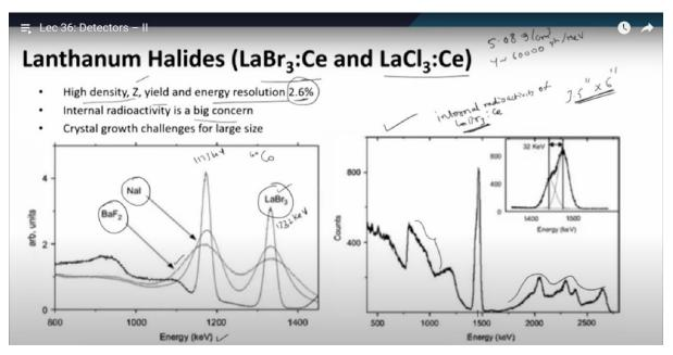
Of course, sometimes we are interested in measuring the angular correlation between these two gamma rays as well. But here in the spectrum of barium fluoride, sodium iodide and lanthanum bromide you can see. Lanthanum bromide supersedes sodium iodide which supersedes barium fluoride. So, the advantage of barium fluoride is basically it has a high density. So, its efficiency is higher than the sodium iodide but resolution is very poor.
