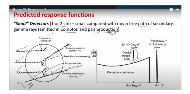
And this emits 511 keV gamma rays in both directions. So, this we are calling as escaping annihilation photons. And here the response of the crystal if it is less than the 2 m 0 c square and more than 2 m 0 c square. One should be able to draw the spectrum. So, when I say energy spectrum what does it mean? It is the distribution of energy of the gamma rays. So, when I say spectrum, it is the distribution of energies.
