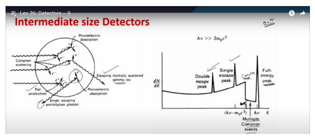
So, what is this? Because of the multiple Compton scattering other than theta is equal to pi energy corresponding to theta is good pi. If it undergoes Compton scattering again it can deposit more energy. And that comes in between Compton edge and full energy peak. And due to multiple Compton scattering if full energy is deposited like in instalment but full energy is deposited. It comes under the photo peak. So, now this peak is no more because of the photoelectric effect.
