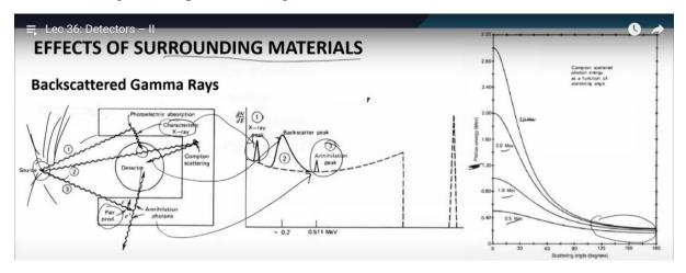
And scattered gamma ray can come back to the detector. So, all these scenarios are possible and if the energy is sufficiently high it can undergo pair production within the surrounding material. And it can emit annihilation photons and these photons can enter into the detector. So, there is always a good possibility that detector detects the radiation not only from the source but also the radiation emitted by the surrounding materials.
