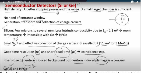
So, let us discuss more about the semiconductor detectors. So, the density is of course higher than the ionization chambers. So, I am comparing with now ionization chambers, gas field detectors. So, because of the high density the stopping power is also good, that means dE by dX. The energy loss per unit length is also quite high. So, the range is very small. So, one can have small size detectors and there is a possibility to go for small target chamber.
