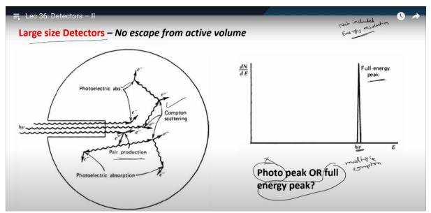
multiple Compton scattering also. And you have for in photo I mean pair production also it is giving rise to the emission of 511 keV gamma rays which are again deposited within the crystal.
