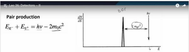
And in pair production you know the energy of the electron and positron should be in such a way that it is equal to the incident energy - two 511 keV gamma rays. So, that is the reason you will get a peak which is left to the full energy by an amount of 2m0c square. This is also called as double escape peak.
