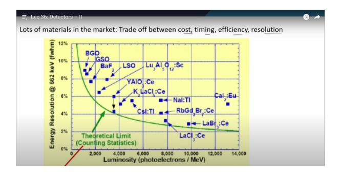
So, there are lots of materials in the market. There is a trade-off between cost, timing, efficiency and the resolution and there is a theoretical limit. No crystal could reach the theoretical limit like lanthanum bromide, which little bit comes to this theoretical limit and lanthanum chloride. And one crystal is there YAIO3 Ce this comes after certain conditions close to the theoretical limit in terms of resolution.
