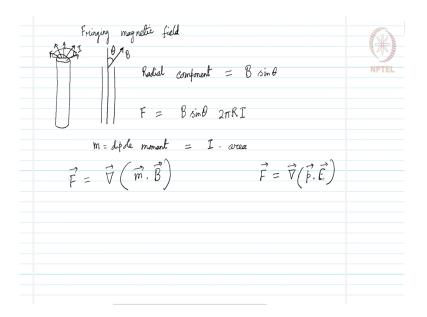
So, if we consider a finite solenoid like this, this is an end this is another end. So, here at this end the magnetic field would point along these directions; something like this and these are the fringing magnetic fields.
