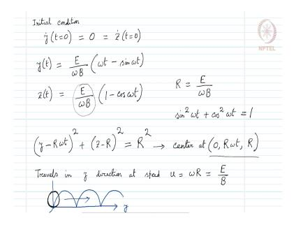
So, the initial condition can be written down as y dot at t equals 0 is 0 there is no velocity along any direction. So, z dot at t equals 0 is also 0 and the particle is at the origin. So, y and z those are also 0 at t equals 0. Now, if we apply this initial condition on the general solutions for the differential equations, we will find the specific solution to this problem y t equals E over omega B omega t minus sin omega t and z t would be given as E over omega B one minus cosine of omega t.
