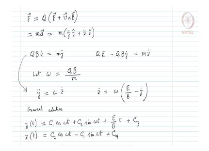
Now, we can write down the equation of motion as using the second law of motion force equals the charge times the electric field plus velocity cross the magnetic field. That means, mass times the acceleration equals this quantity is also equal to mass times the acceleration that is mass times y double dot in y direction plus z double dot in z direction.
