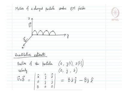
So, this time we are considering motion of a charged particle under electromagnetic force under the influence of electromagnetic fields. So, as a simple example let us consider that the magnetic field points along x direction and electric field points along the z direction.
