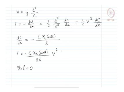
So, we will have to write this expression for energy stored in the dielectric, energy stored in the capacitor in terms of the conserved quantity namely total charge that is half Q squared over the capacitance.
