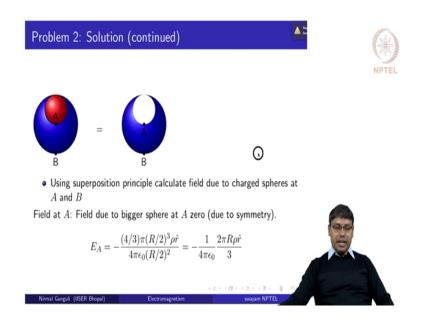
So, after doing this so; that means, this situation is equivalent to this situation that is that we are given with. So, we can find the electric field corresponding to this situation. By applying this principle of superposition on this situation and applying principles of superposition on this principle this situation is much easier using principle of superposition now you can calculate the electric fields at point A and point B.
