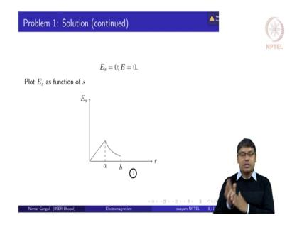
Now, comes the last part of the problem that is plotting E s as a function of s the plot could look something like this. Initially, the value of E s will linearly increase with increasing s and then it will decay as 1 over s up to r equals b; beyond r equals b we are coming outside of the coaxial cable and outside of the coaxial cable there is no electric field at all.
