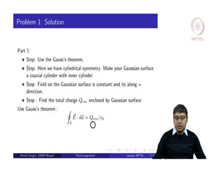
Let us go through the solution. In part 1, the steps to solve the problem is first you have to use the Gauss's theorem. Here we have cylindrical symmetry. So, make your Gaussian surface a coaxial cylinder with the inner cylinder. And in the first one we will have the inner Gaussian surface inside the inner cylinder.
