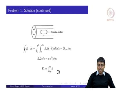
How do we do that? So, here we have shown a Gaussian surface inside the inner cylinder and the length of this Gaussian surface cylinder is 1. So, we will have a closed integral over E dot da given as integration from 0 to 1 over z that is the length of this Gaussian surface. And integration over 0 to 2 pi over phi that is the azimuthal angle that we have E s times r cap dot r cap; s d phi d z and that will give us total charge enclosed over epsilon naught.
