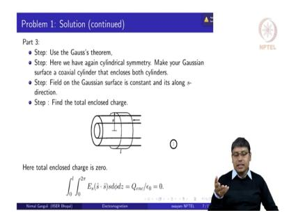
And in the part 3, we are supposed to find the electric field outside everything outside the entire coaxial cable. Again the method would remain the same, you are supposed to apply Gauss theorem you are supposed to consider the cylindrical symmetry and make a cylindrical Gaussian surface coaxial with the cylinder and that enclose both cylinders.
