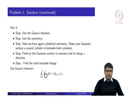
And in the second part, we are supposed to find the electric field in between the cylinders. So, there we have to consider again the Gauss Gaussian the Gauss theorem, we have to consider the symmetry and we need again a cylindrical Gaussian surface. And this time this Gaussian surface will enclose the smaller cylinder but it will not enclose the larger cylinder; it will lie somewhere in between the cylinders; that means, it will be inside the coaxial cable.
