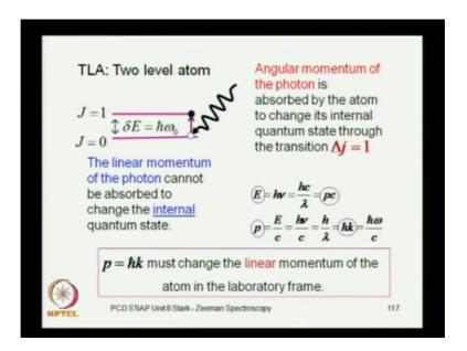
And to understand this process of cooling, we consider a two level atom, so let us consider a two level atom in a stage J is equal 0. And it is absorption of photon could raise it to J equal to 1 at exited state, and let us say that light falls on it, resonant light which is appropriate for this transition from the lowest state to the exited state, and the atom gets exited.
