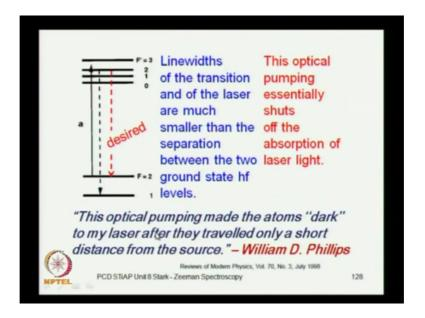
And actually, it towards to come down to the same level, you could re pump, and then you would have an appropriate cooling cycle, but in the absent of that. Since, it decay or it has the possibility of decay to a different level, then you not have the appropriate cooling cycle available. So, the line width of the transition of course, are much smaller than the differences between these energies, that we have taken for this, it is not the case over here.
