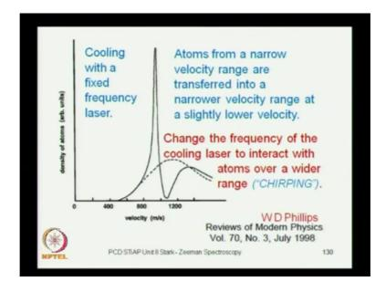
So, using the re pump he is using to get a good amount of laser cooling achieve, what essentially is happening is that atoms very the narrow velocity range, are transferred in to a narrower range. And you gradually step by step tell you really achieve a lot of cooling, so this is to be done using chirping is one way of doing it, so adjusting the frequency of the cooling laser.
