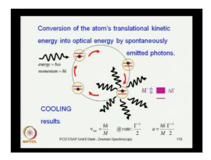
So, this is how cooling results what is happening is that the atoms translational kinetic energy, gets converted into optical energy through spontaneous emission of photons, so there is an energy transform through this process. So, this is like taking an additional degree of freedom into account, which was not there originally which is losing light through to the surrounding.
