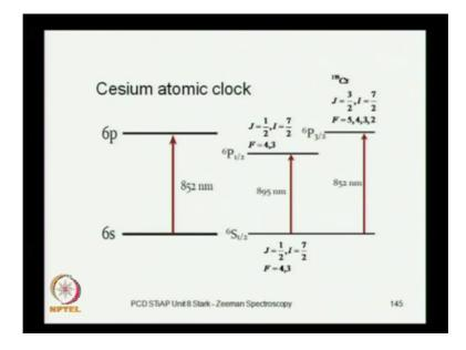
The cesium atomic clock comes 6 s to 6 p which has brought a fine structure, and then hyperfine structure coming from the nucleus spin, which is 7 half. So, the 6 p 3 half state gives you additional levels gives you this quadrate, with F equal to 4 5 4 3 and 2 coming from the combination of these two angular of momentum. And then the 6 p 1 half states, gives you this F equal to for and 3 double it and the lowers states is also double it with the F equal to 4.
