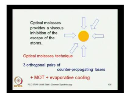
That these is an optical molasses, in which you inhabit the escape of the atom out of these zone, so that is the reason this is called optical molasses. Then you do use additional you know techniques like magnetic optical traps, and then you also exploit what is called as a evaporative cooling, you know what evaporative cooling is that if you have a hot cup of tea over here.
