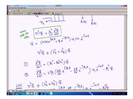
We wanted to find out this wave equation for fiber Bragg grating and psi was in total A function of z e to the power of i beta 1 z plus B e to the power of minus of i beta 1 z psi 1 which is a function of x and then e to the power of minus i omega t, that was the by definition that was the psi.
