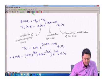
Now, I can construct in detail that, big psi which is a function of x and z can be written as psi f plus psi b already mentioned; this psi f, psi b also function of x and z. So, psi f which is a function of x and z is defined as a amplitude term; we already mentioned that, this amplitude term should be function of z, should be function of z, mind it this is z direction. And then e to the power of i forward propagation constant beta 1 z minus omega t and the transverse field.
