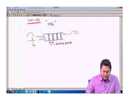
FBG in short Fiber Bragg Grating. So, quickly want to remind what is the principle of fiber Bragg grating that, we have a grating structure inside the fiber core that is the first thing. And
