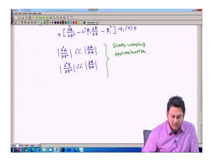
And also del 2 B del z square. So, we considered that the amplitude is varying over z and this variation is a slow variation; that is why the second order derivative with respect to z I can neglect compared to the first order derivative. So, this is called the slowly varying approximation. So, if I make a slowly varying approximation, then what happened; this equation will be little bit simplified.
