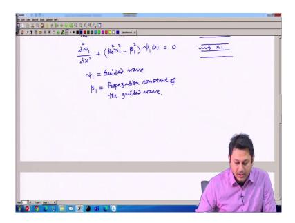
And beta 1 was the propagation constant of the guided wave, ok. Now, for FBG what happened that we have some kind of modulation here in the core region, it is not n 1; but on top of that we have a modulation and this modulation we already wrote here, n 1 square plus some modulation is there and that modulation is due to the fiber Bragg gating, because the grating is now there.
