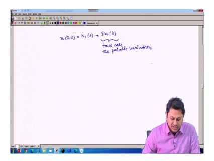
So, refractive index variation in the last class we defined, now it is a function of x and z. So, this is a refractive index of the core, original refractive index of the core without any kind of perturbation and delta n is a variation or this is the perturbation we have. And this is basically the, this basically takes care; this delta n basically take care the periodic variation of the refractive index.
