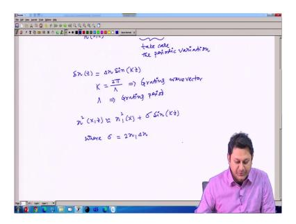
Now, these delta n which is a function of z; since it is taking care of the periodic variation, so I can write it as a periodic variation like that, where K which is equal to 2 pi divided by big lamb the period of the grating is called the grating wavelength, this is called the grading wavelength, we will define that later.
