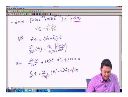
So, my wave equation is grad square psi is equal to n square c square d 2 big psi d t square. Now, one by one we calculate, where grad square big psi; let us calculate the left hand side first, left hand side, which is equivalent to this, d 2 x plus d 2 z, this one. D 2 d x square if I now calculate one by one big psi, so this is the first term.
