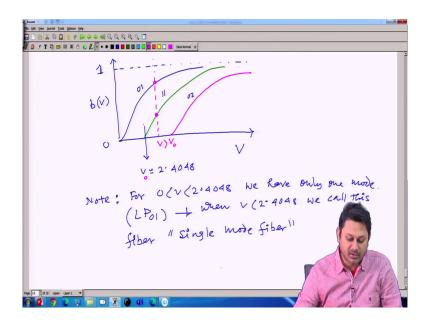
So, I can have the value of b. So, I can plot that like we have done in the previous case, we can plot this. This is again a well-known plot. So, 0, this is 1. Along this direction, I plot b as a function of V. And I am going to have this kind of curves. So, along this direction, I am plotting V, increasing V.
