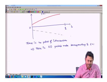
Now, for this same V value if I plot for same V value, if I plot this equation for I equal to 1, initially it is for I equal to 0, now I am plotting for I equal to 1. I am going to have two function like this. This side I am plotting b which is 0 which is restricted up to 1, and this is 1. And when I plot, there is no cutting point at all.
