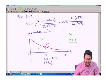
So, for suppose for I equal to 0, what happened? I have the transcendental equation V 1 minus b whole to the power half J 1 V 1 minus b divided by J 0 V 1 minus b. This is my left hand side of the transcendental equation. And the right hand side, I have V root over of b K 1 V root b divided by K 0 V root b.
