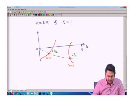
If I do, so say V equal to 6.5, and you can see the value of V is much greater than 2.40 this cut off. So, we are going to expect more than one mode to be supported by the fiber and I equal to 1.
