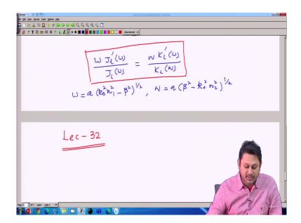
Well, in the last class if you remember, we had a transcendental equation like this after putting a second boundary condition. And then we mention that if I able to solve this equation, then I can find out what is the value of this beta which is important which is basically the propagation constant of a given mode.
